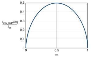
Figure 2. I<sub>CIN</sub> vs. Voltage Conversion Ratio
