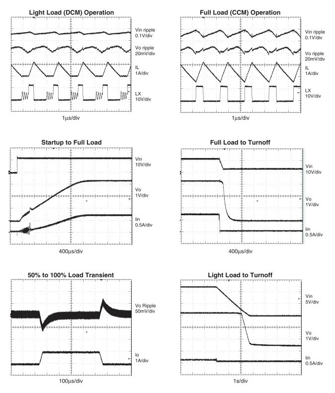
**Typical Performance Characteristics** *(Continued)* Circuit of Figure 1.  $T_A = 25^{\circ}C$ ,  $V_{IN} = V_{EN} = 12V$ ,  $V_{OUT} = 3.3V$  unless otherwise specified.
