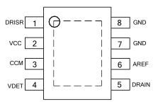
Note: The DRAIN pin of internal MOSFET is exposed PAD, which is at the bottom of IC (the dashed box). The secondary current should flow from GND(pin 7,8) toth is exposed PAD.
