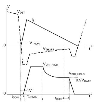
Figure 1. Typical Waveforms of APR34509 in DCM
