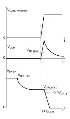
Figure 2. Typical Turn Off Waveforms of APR34509 in CCM
