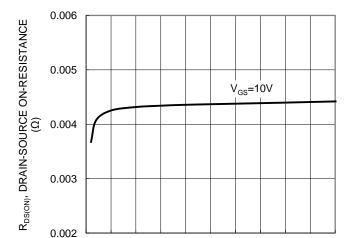
${\rm I_D}, {\rm DRAIN\text{-}SOURCE}$  CURRENT (A) Figure 3. Typical On-Resistance vs. Drain Current and Gate Voltage
