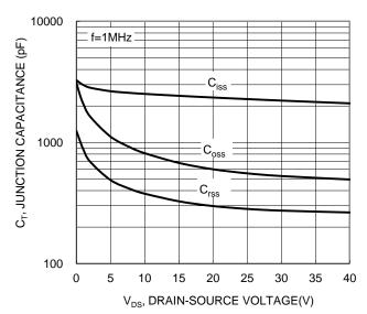
Figure 11. Typical Junction Capacitance
