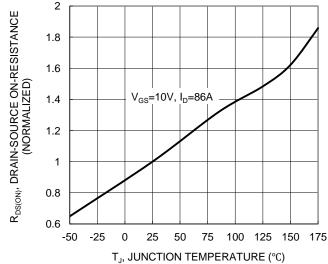
Figure 6. On-Resistance Variation with Junction
