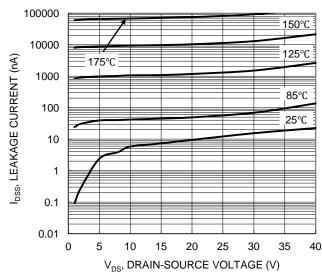
Figure 10. Typical Drain-Source Leakage Current vs.
