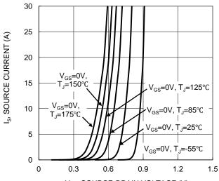
V<sub>SD</sub>, SOURCE-DRAIN VOLTAGE (V) Figure 9. Diode Forward Voltage vs. Current
