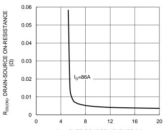
V<sub>GS</sub>, GATE-SOURCE VOLTAGE (V) Figure 4. Typical Transfer Characteristic
