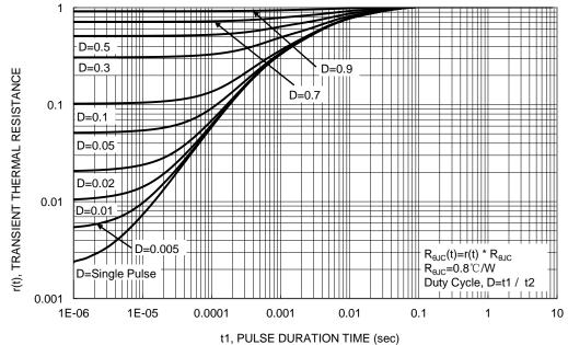
Figure 14. Transient Thermal Resistance
