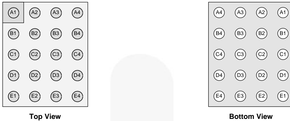
Figure 4. WLCSP-20 Pin Assignments
