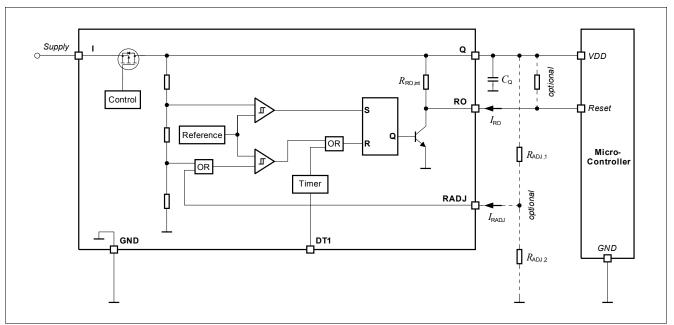
Figure 6 Block Diagram Reset Circuit
