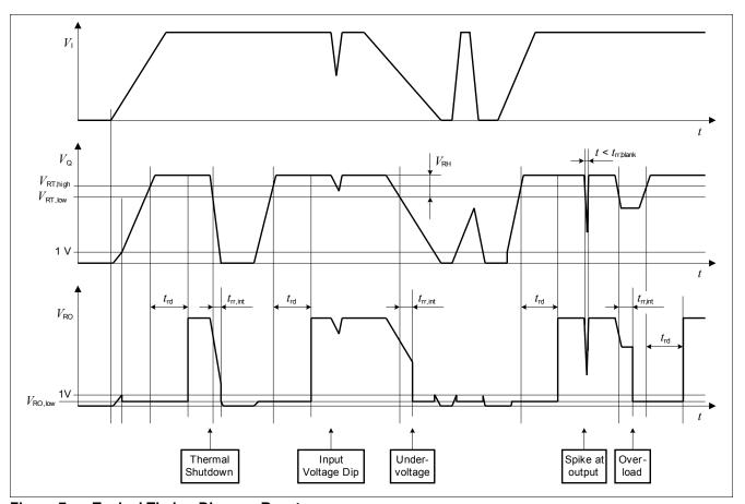
Figure 7 Typical Timing Diagram Reset
