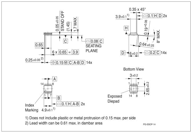
Figure 14 PG-SSOP-14
