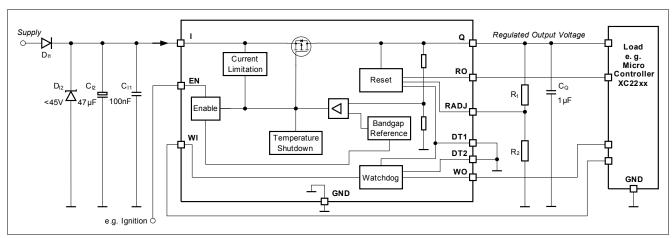
Figure 13 Application Diagram
