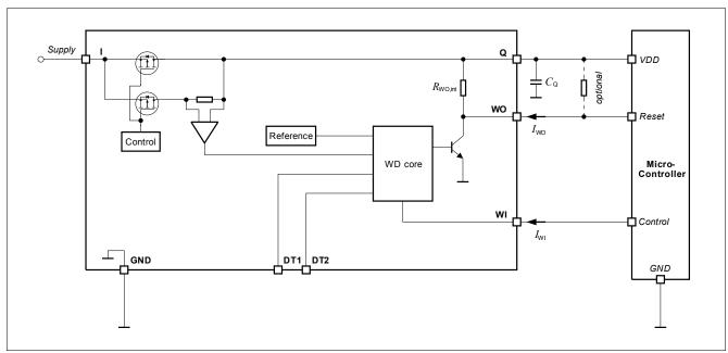
Figure 8 Block Diagram Watchdog Circuit
