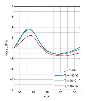
Output Voltage  $V_{\rm Q}$  versus Input Voltage  $V_{\rm I}$  (5 V version)
