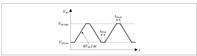
Figure 10 Test Pulses Watchdog Input WI
