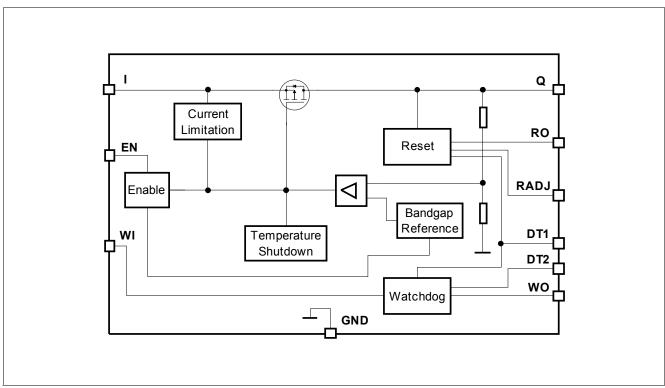
Figure 2 Block Diagram TLS820F0ELV50 and TLS820F0ELV33
