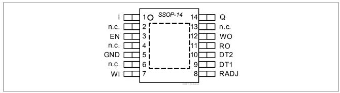
Figure 3 Pin Configuration
