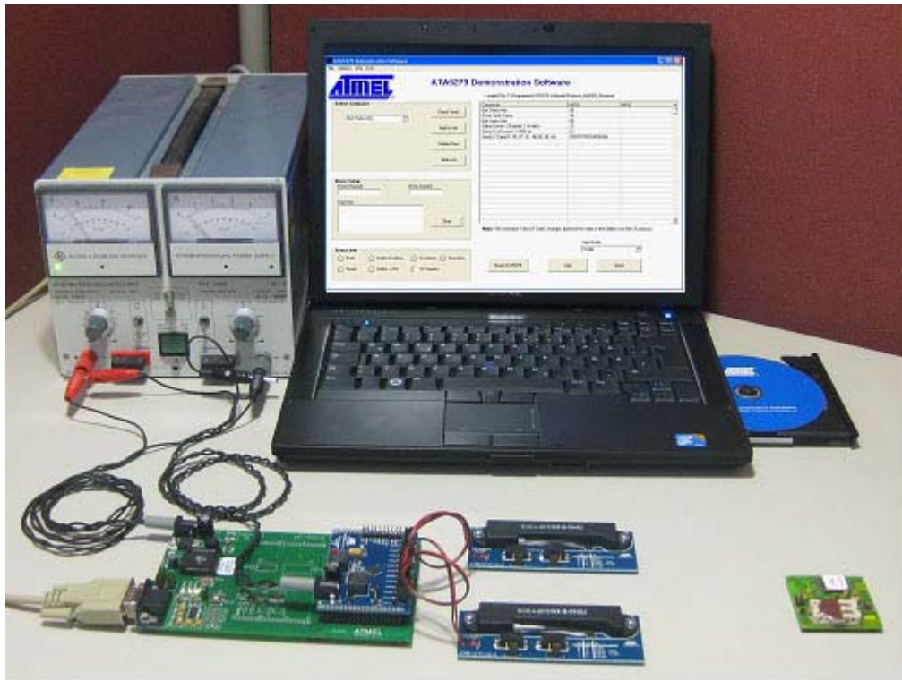
Figure 1-1. LF Wake-up Demonstration System
