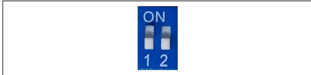
FIGURE 3-1: SW9 IN FLASH APPLICATION MODE
