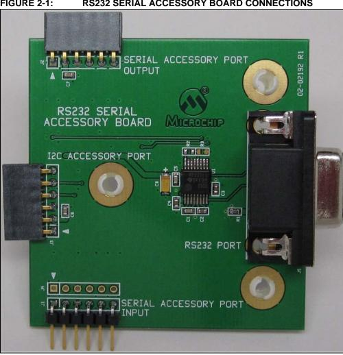
FIGURE 2-1: **RS232 SERIAL ACCESSORY BOARD CONNECTIONS**
