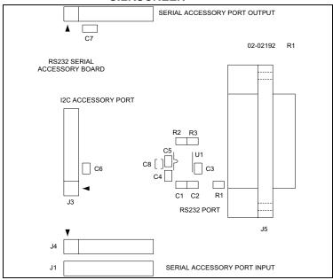
Figure A-2 illustrates the RS232 Serial Accessory Board top copper.
