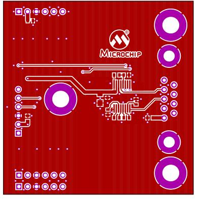
Figure A-4 illustrates the RS232 Serial Accessory Board bottom copper mirrored.
