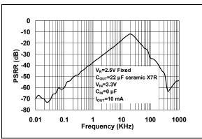
**FIGURE 2-26:** Power Supply Ripple Rejection (PSRR) vs. Frequency (V<sub>OUT</sub> = 2.5V Fixed).
