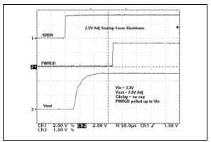
**FIGURE 2-28:** 2.5V (Adj.) Startup from Shutdown.
