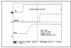
FIGURE 2-27: 2.5V (Adj.) Startup from V<sub>IN</sub>.
