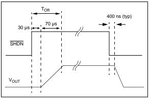
FIGURE 4-5: Shutdown Input Timing Diagram.
