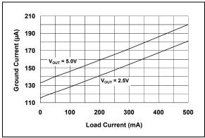
**FIGURE 2-12:** Ground Current vs. Load Current.
