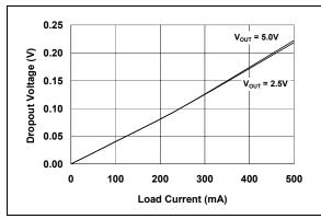
FIGURE 2-19: Dropout Voltage vs. Load Current.
