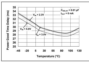
**FIGURE 2-9:** Power Good (PWRGD) Time Delay vs. Temperature (Adjustable Version).
