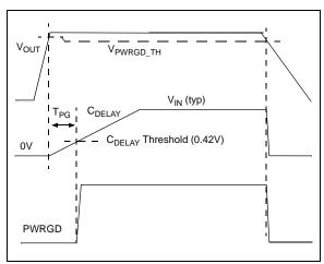
**FIGURE 4-4:** C<sub>DELAY</sub> and PWRGD Timing Diagram.
