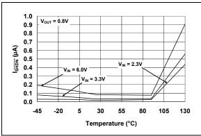
FIGURE 2-14: I<sub>SHDN</sub> vs. Temperature.
