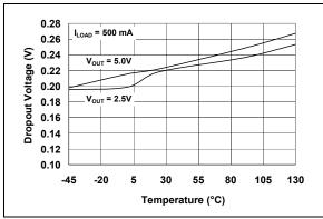
**FIGURE 2-20:** Dropout Voltage vs. Temperature.
