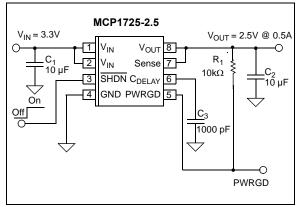
FIGURE 5-1: Typical Application Circuit.
