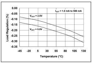
**FIGURE 2-18:** Load Regulation vs. Temperature ( $V_{OUT} \ge 2.5V$  Fixed).
