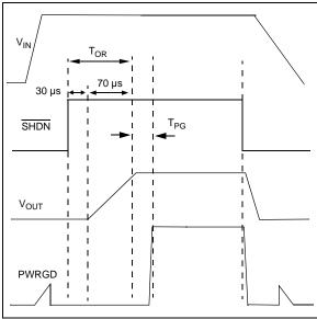
**FIGURE 4-3:** Power Good Timing from Shutdown.
