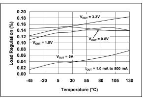
FIGURE 2-5: Load Regulation vs. Temperature (Adjustable Version).
