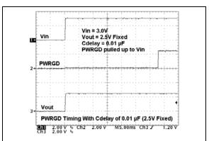
FIGURE 2-30: Power Good (PWRGD) Timing with C<sub>DELAY</sub> of 0.01 μF (2.5V Fixed).
