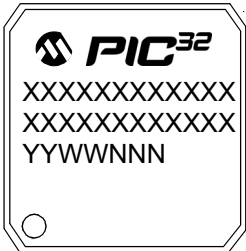
100-Lead TQFP (14x14x1 mm)
