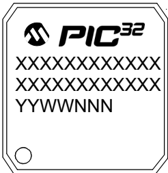
100-Lead TQFP (12x12x1 mm)
