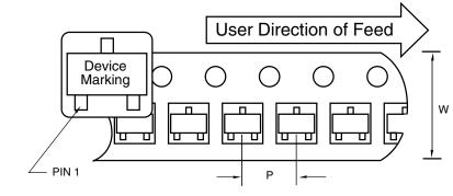
Standard Reel Component Orientation For TR Suffix Device (Mark Right Side Up)
