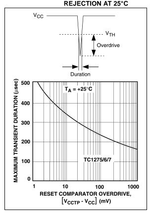
FIGURE 3-6: ENSURING RESET VALID TO  $V_{CC} = 0V$
