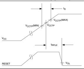
FIGURE 3-4: Timing Diagram – Power Down (TC1277)
