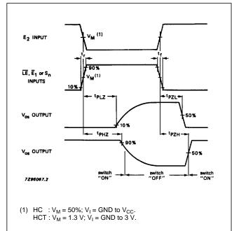
Fig.19 Waveforms showing the turn-ON and turn-OFF times.
