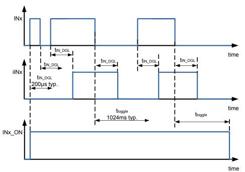
Figure 35. IN, iIN and IN\_ON signal
