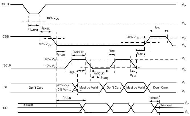
Figure 8. Timing Requirements During SPI Communication
