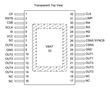
Figure 3. 12XS6 Pinout Diagram
