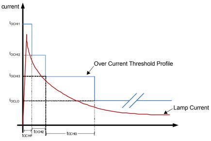
Figure 15. Transient Overcurrent Profile
