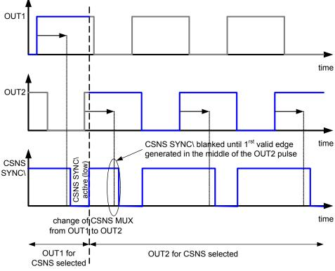
Figure 32. CSNS SYNCB TRIG1/2 Setting
