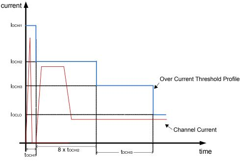
Figure 19. HID Ballast Overcurrent Profile
