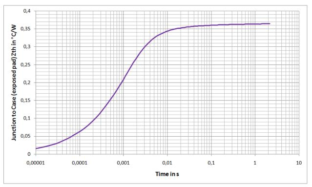
Figure 38. Transient Thermal Response Curve
