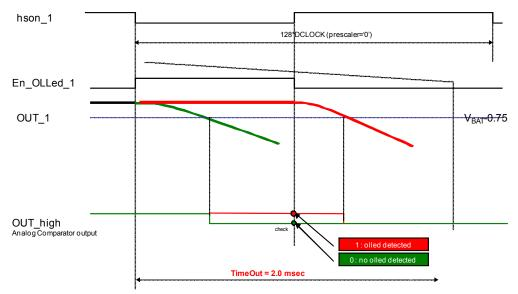
Figure 24. Open Load in ON State for LED in PWM Operation (OFF time < 2.0 ms)
