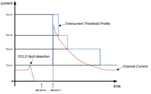
Figure 17. Resetable Overcurrent Profile
