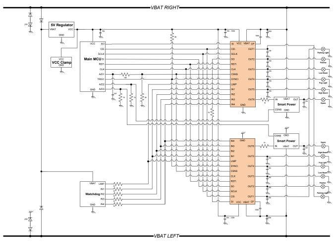
Figure 36. Typical Automotive Front Lighting
