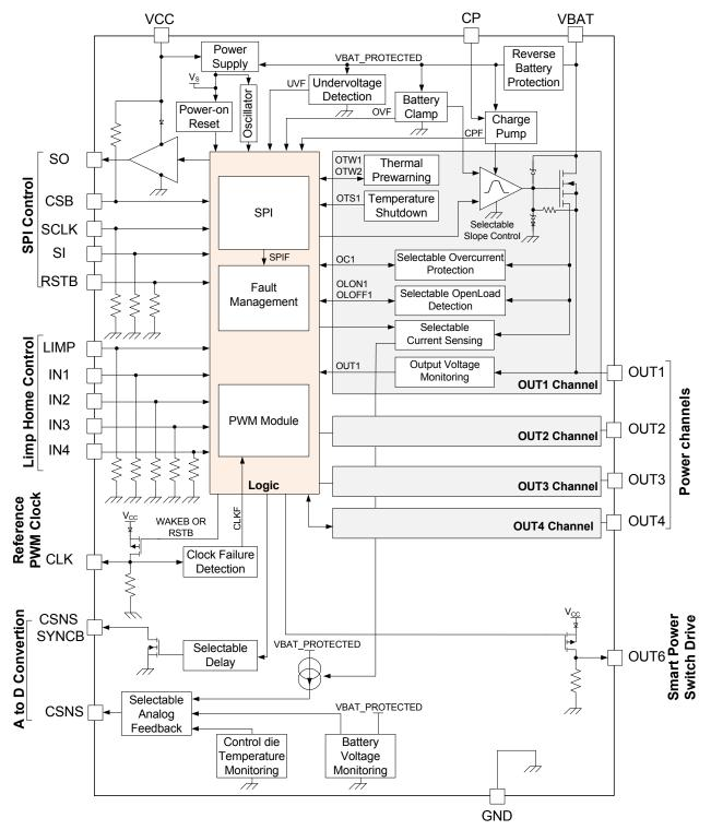
Figure 2. Simplified Internal Block Diagram (Quad version)
