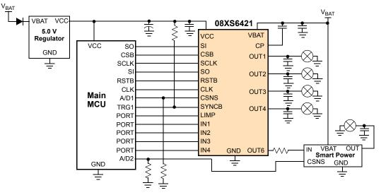
Figure 1. Dual 8.0 m $\Omega$  and Dual 21 m $\Omega$  Simplified Application Diagram
