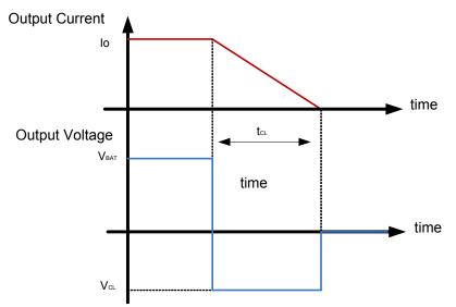
Figure 21. Simplified Negative Output Clamp Waveform
