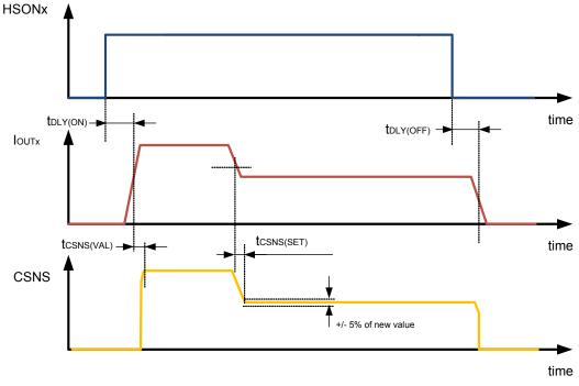
Figure 27. Current Sensing Response Time
