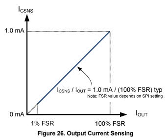
The feedback is suppressed during OCHI window ( $t \le t_{OCHI1} + t_{OCHI2} + t_{OCHI3}$ ) and only enabled during low overcurrent shutdown threshold (OCLO). During PWM operation, the current feedback circuit (CSNS) delivers current only during the on time of the output switch. Current sense settling time,  $t_{CSNS(SET)}$ , varies with current amplitude. Current sense valid time,  $t_{CSNS(VAL)}$ , depends on the PWM frequency (see Electrical Characterization).
