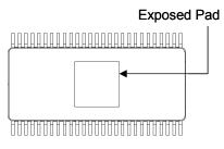
Figure 2. 54Id SOIC-EP Backside View
