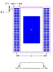
Figure 6. SOIC Land Pattern Dimensions
