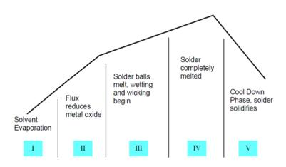
Figure 18. General Solder Reflow Phases
