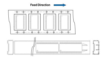
Figure 17. SOIC Orientation in Tube and Tape & Reel
