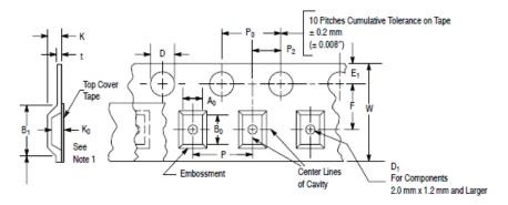
Figure 24. Carrier Tape Specifications
