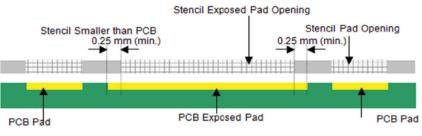
Figure 15. Reduced Solder Stencil Aperture for Exposed Pad
