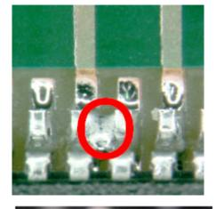
Foreign Matter Under SOIC Causing Open Corner Leads
