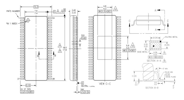
Figure 4. Example of SOICW 54LD Case Outline Drawing
