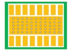
0.3 mm Diameter at 1.2 mm Pitch Thermal Via
