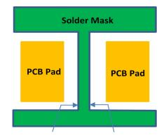
Figure 13. Pad and Solder Mask with Thin Webbing
