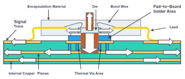
Figure 7. Cross-Section of EP Package with Heat Transfer Schematic
