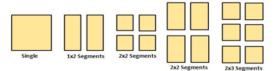
Figure 16. Segmented Stencil Openings
