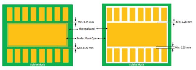
Figure 8. Example of Exposed Pad Land Pattern
