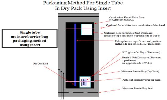
Figure 22. Sample of Single Tube Packing Method
