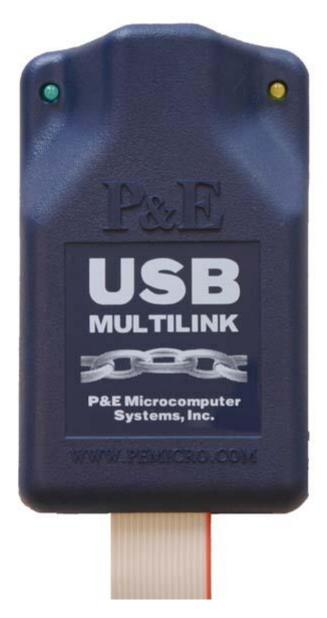
The MON08 Multilink is an easy-to-use, low-cost development tool for Freescale's 68HC08 flash MCUs. The MON08 Multilink provides in-circuit emulation, debugging and programming through the 68HC08's standard MON08 serial debug/breakpoint interface.
