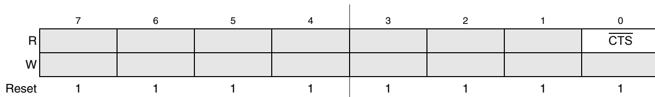
Figure 15-20. Input Port Register (UIP n )
