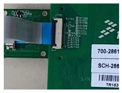
Figure 11. Connect the BT module
