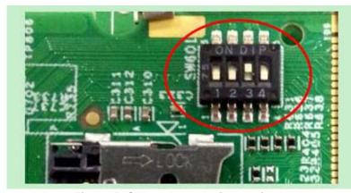
Figure 5. SW601 boot device settings
