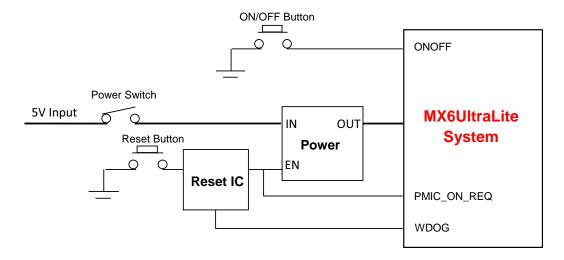
Figure 9. Power Control Diagram
