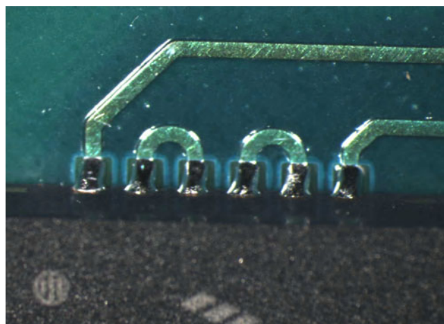
Figure 11. No Solder Balling was Observed for Case 6L-C, d = 0.40 mm, Sn62 Solder (Good Fillets Formed Above the Extended Part of PCB Pads)
