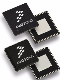
Figure 5. Singulated QFN. Top: Saw Bottom: Punch
