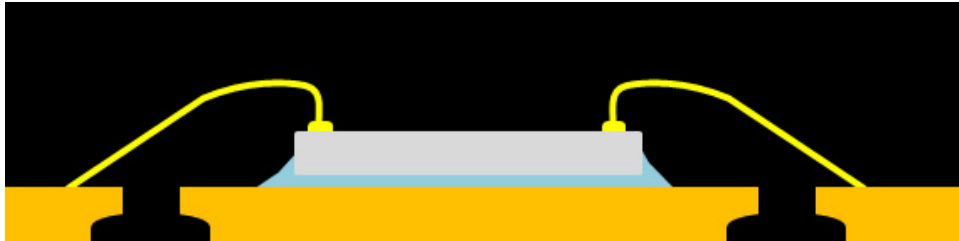
Figure 2. Sawn DFN/QFN (Cross-section View)
