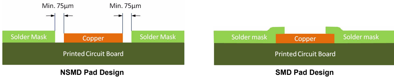
Figure 16. NSMD and SMD Pad Designs
