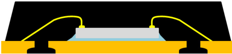
Figure 3. Punch QFN (Cross-section View)
