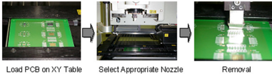
Figure 32. Package Removal Process
