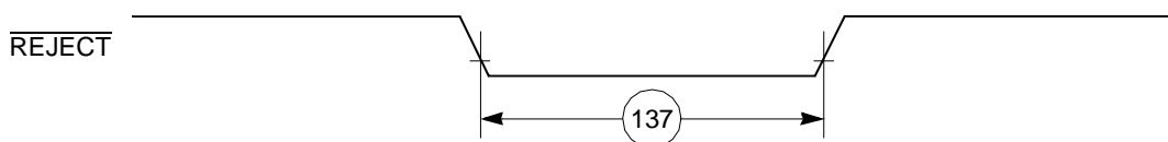
Figure 54. CAM Interface REJECT Timing Diagram
