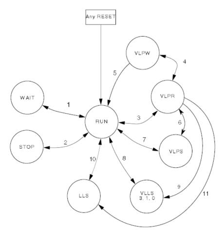
Figure 6. Power mode state transition diagram
