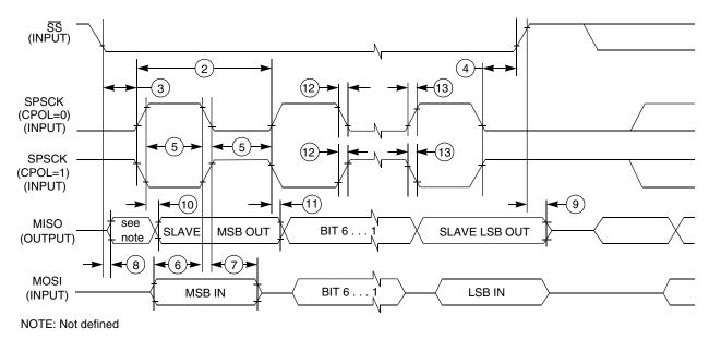
Figure 15. SPI slave mode timing (CPHA = 1)
