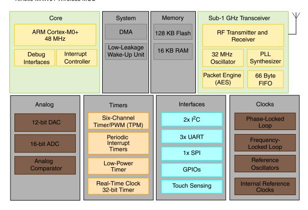
Figure 1. MKW01 Simplified Block Diagram
