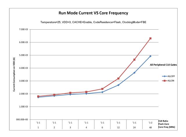
Figure 1. Run mode supply current vs. core frequency
