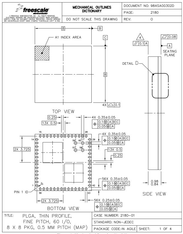
Figure 8. Mechanical Drawing (1 of 2)
