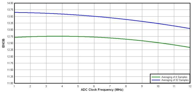
Figure 7. Typical ENOB vs. ADC\_CLK for 16-bit single-ended mode
