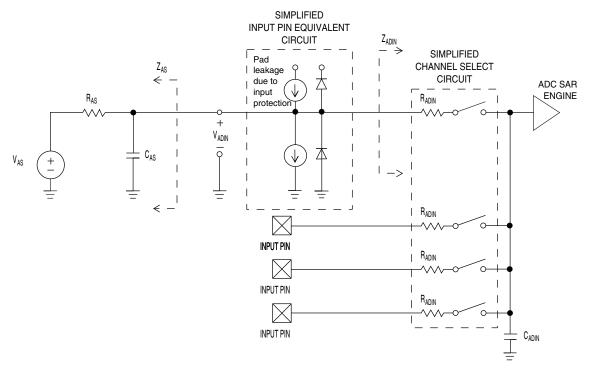
Figure 5. ADC input impedance equivalency diagram
