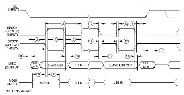
Figure 14. SPI slave mode timing (CPHA = 0)
