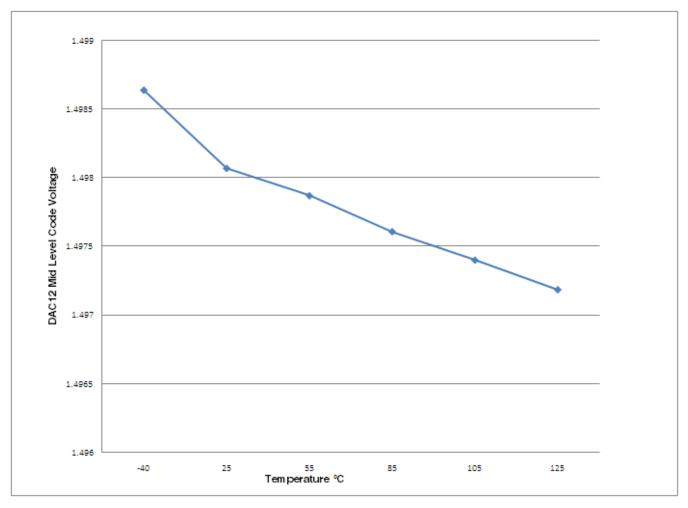
Figure 11. Offset at half scale vs. temperature
