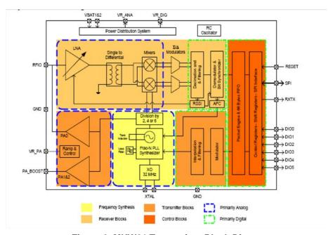
Figure 2. MKW01 Transceiver Block Diagram
