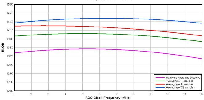
Figure 6. Typical ENOB vs. ADC\_CLK for 16-bit differential mode
