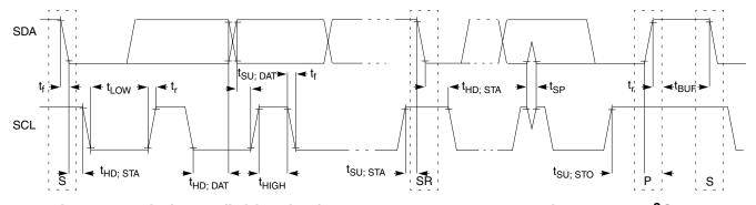
Figure 16. Timing definition for fast and standard mode devices on the I<sup>2</sup>C bus
