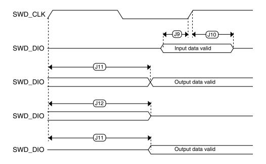
Figure 4. Serial wire data timing
