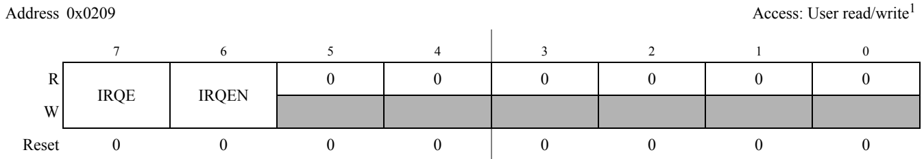
Figure 2-7. IRQ Control Register (IRQCR)
