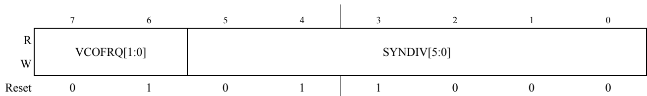
Figure 8-5. S12CPMU_UHV_V7 Synthesizer Register (CPMUSYNR)
