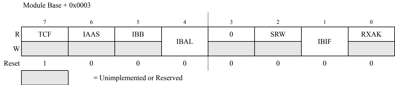
Figure 16-7. IIC Bus Status Register (IBSR)
