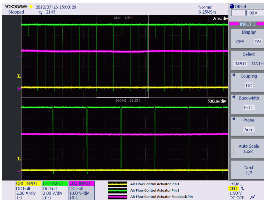
Figure 38. Air flow actuator motor control waveform for defrost position to face & foot position – transition phase
