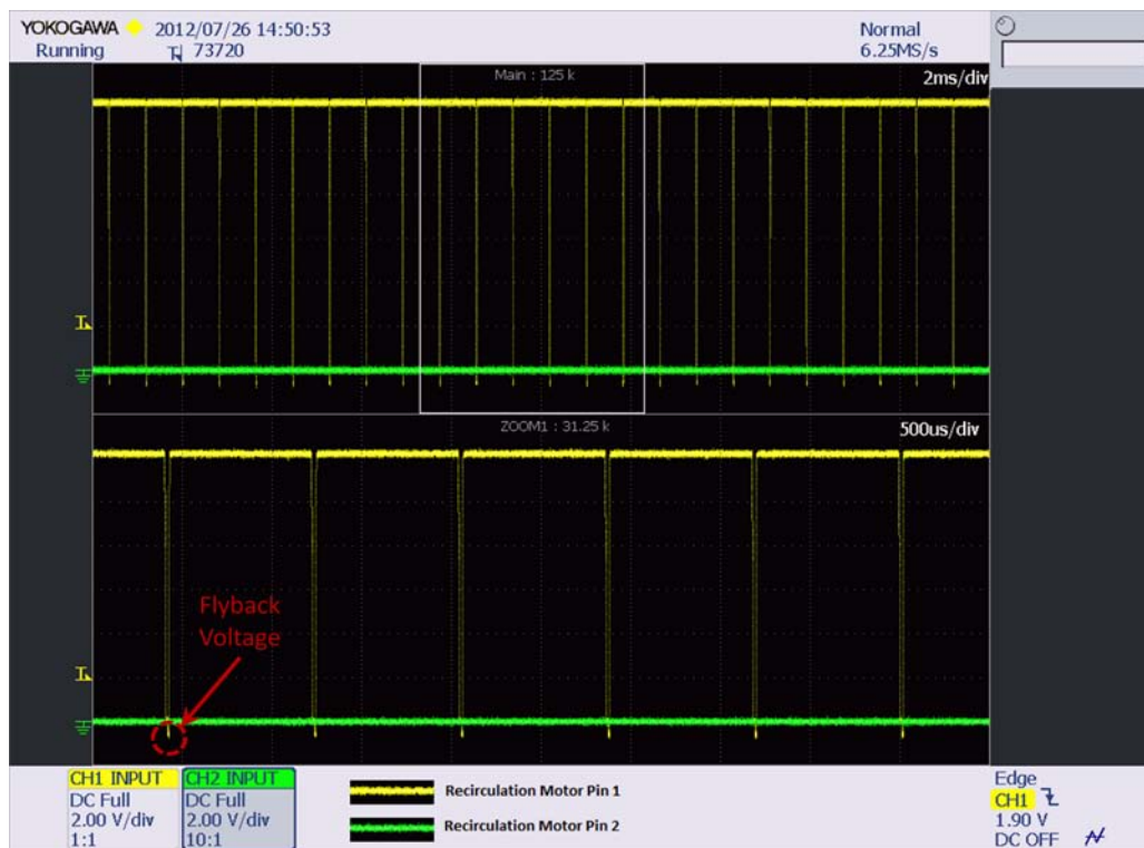
Figure 33. Recirculation motor control waveform for fresh air to internal circulation, when motor is connected
