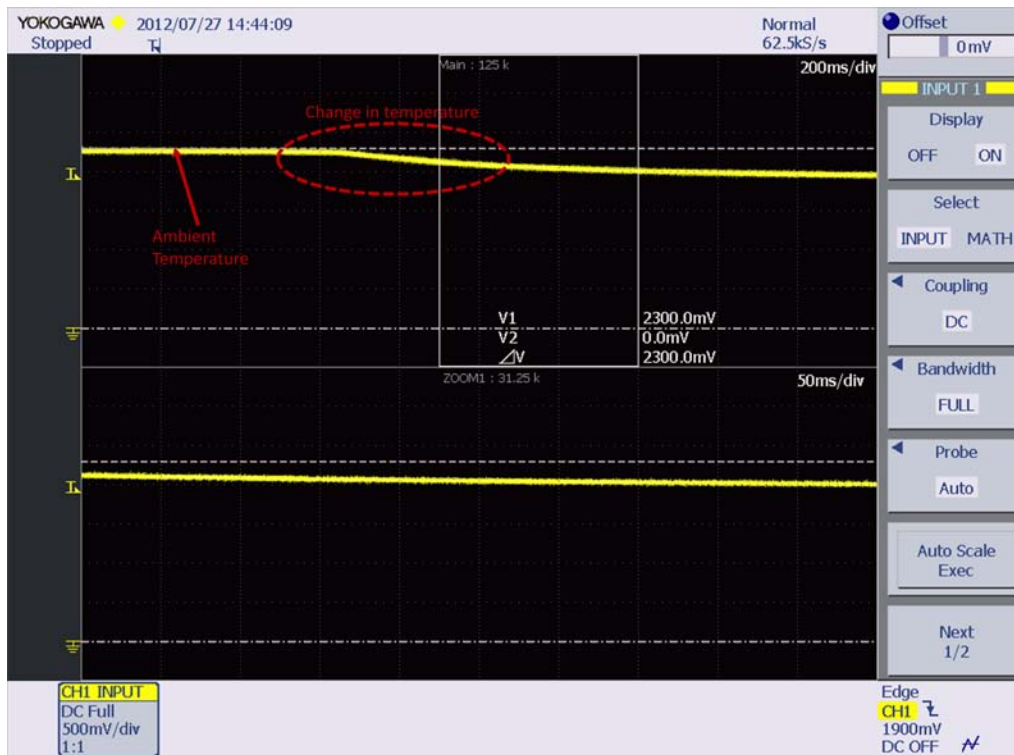
Figure 45. Waveform for temperature sensor output when temperature is increased drastically from the ambient temperature
