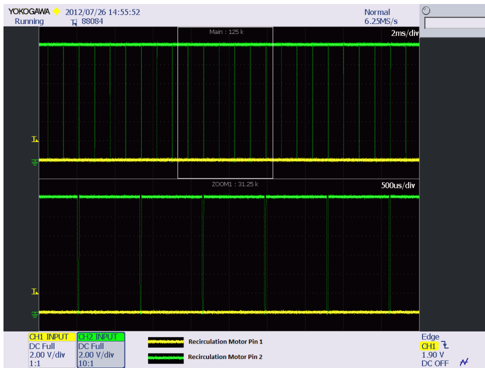
Figure 35. Recirculation motor control waveform for fresh air to internal circulation, when motor is not connected
