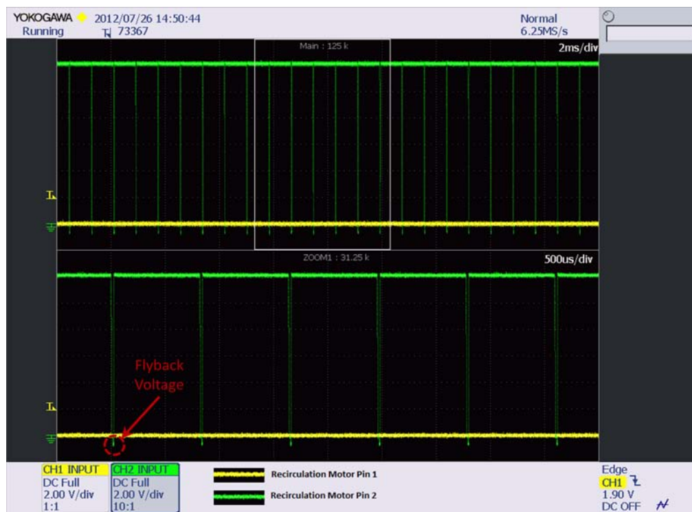
Figure 34. Recirculation motor control waveform for internal to fresh air circulation, when motor is connected
