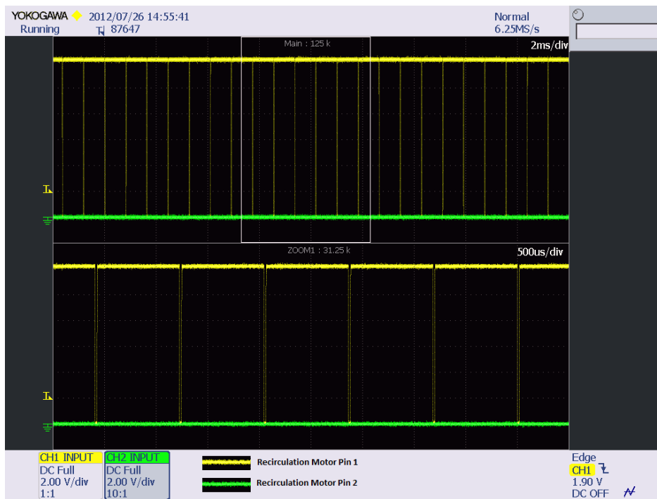
Figure 36. Recirculation motor control waveform for internal to fresh air circulation, when motor is not connected
