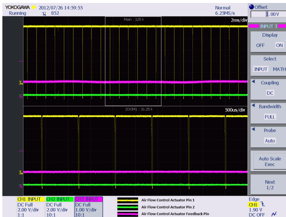
Figure 41. Air flow actuator motor control waveform for face position to foot position – transition phase
