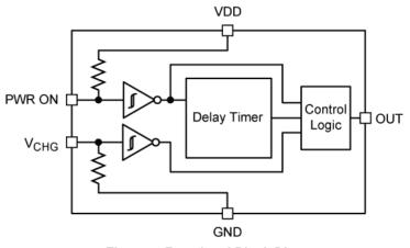
Figure 2. Functional Block Diagram
