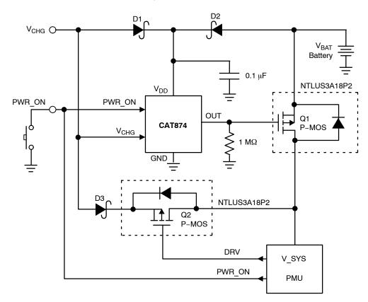
Figure 5. Application Schematic in Dual Supply System
