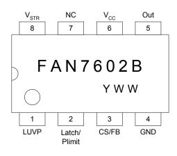
Figure 3. Pin Configuration (Top View)
