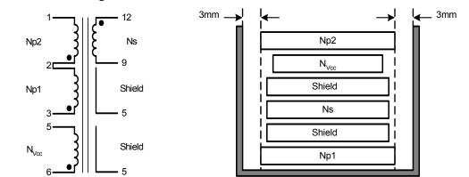
Figure 26. Inductor Schematic Diagram
