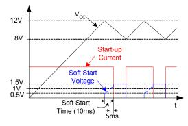
Figure 19. Start-up Current and V<sub>CC</sub> Voltage
