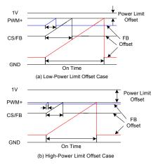
Figure 21. CS/FB Pin Voltage Waveforms
