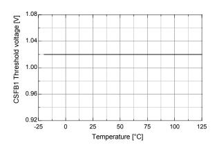
Figure 18. CS/FB Threshold Voltage vs. Temp.
