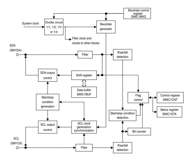
Figure 3.30.1 SMIIC1 Block Diagram
