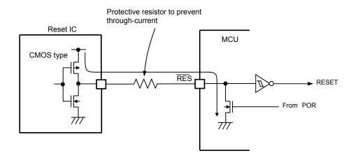
Figure 4-6-7: Example of Reset circuit configuration diagram When using CMOS type
