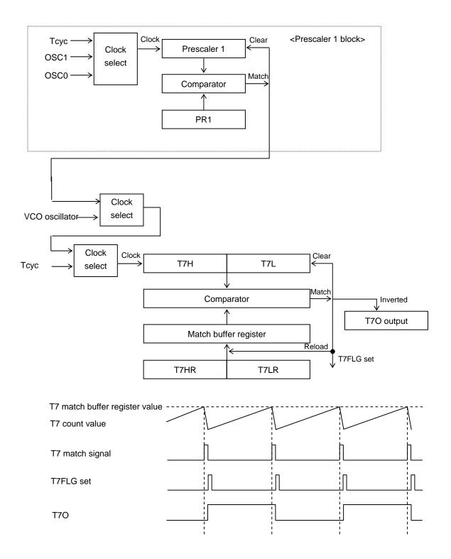
Figure 3.21.2 Timer 7 Block Diagram
