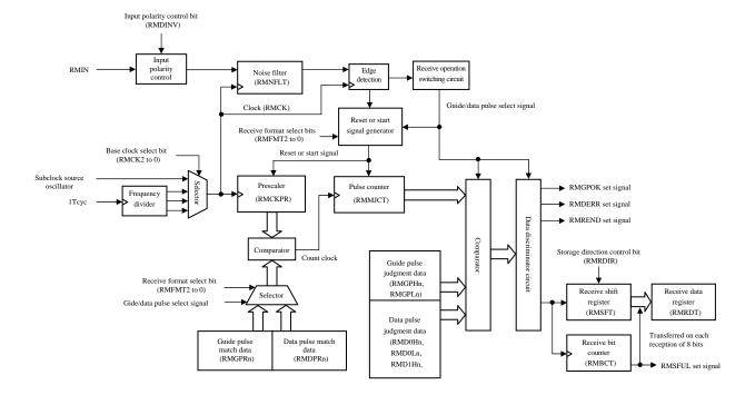
Figure 3.37.1 Infrared Remote Control receiver Circuit Block Diagram
