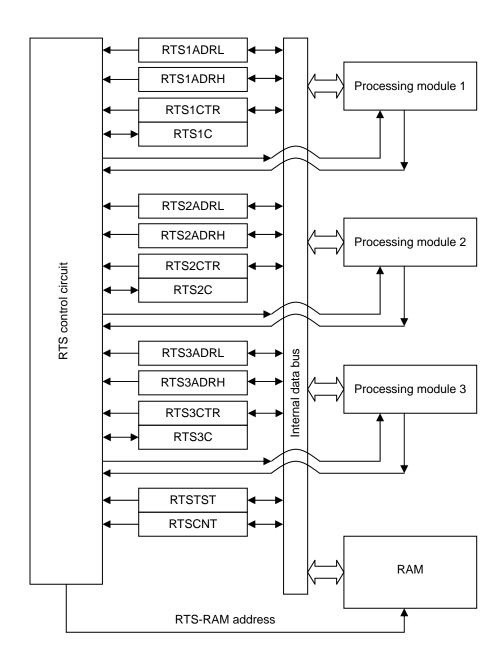
Figure 3.34.1 RTS Block Diagram
