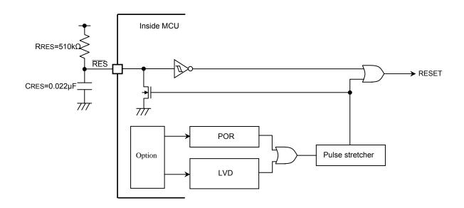
Figure 4-6-1: Internal Reset Circuit configuration diagram
