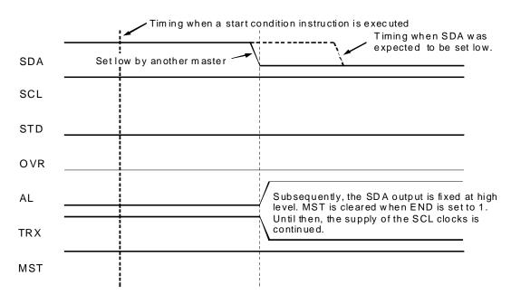
Figure 3.30.10 Arbitration Lost During Start Condition Generation <2>
