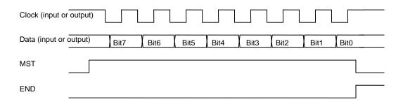
Figure 3.30.11 Waveforms of Simple SIO Mode 1-byte Transmission/Reception
