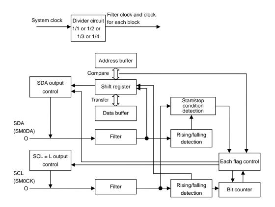
Figure 3.31.1 SLIIC0 Block Diagram
