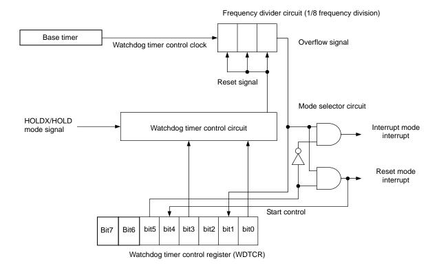
Figure 4.5.1 Watchdog Timer Block Diagram
