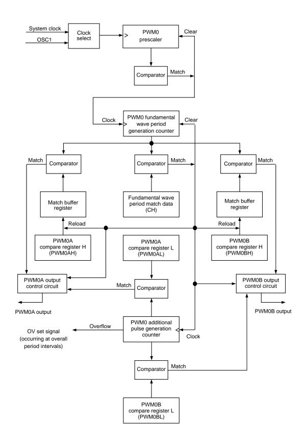
Figure 3.32.1 PWM0 Block Diagram
