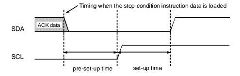
Figure 3.30.7 Stop Condition Generation Timing
