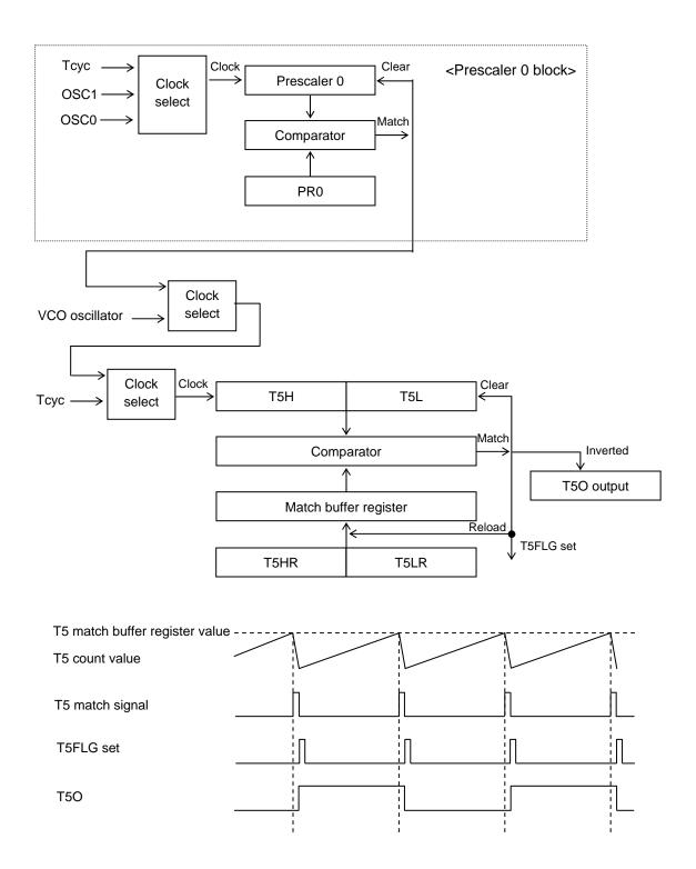
Figure 3.20.2 Timer 5 Block Diagram
