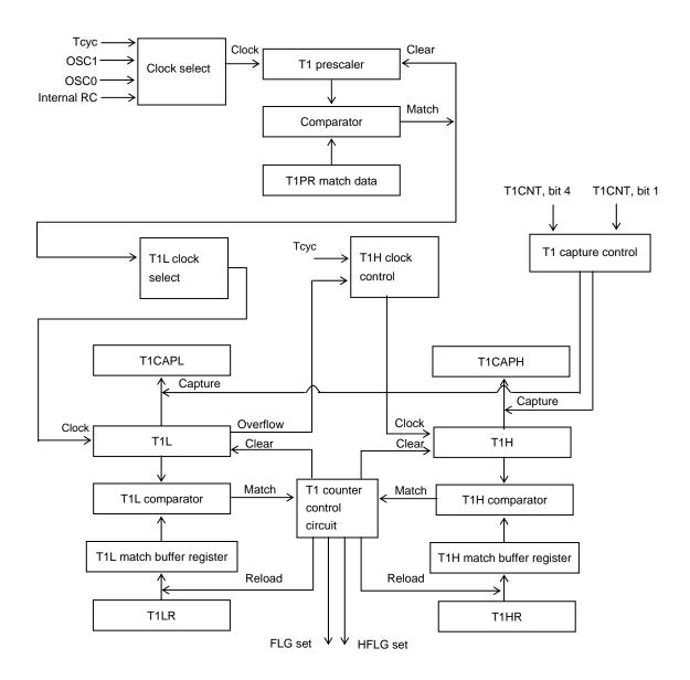
Figure 3.17.1 Timer 1 Block Diagram
