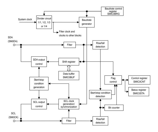
Figure 3.29.1 SMIIC0 Block Diagram
