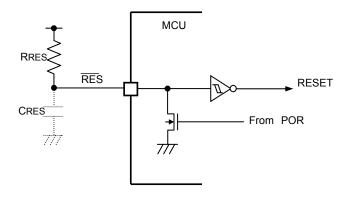
Figure 4-6-2 : Reset circuit configuration example (Internal POR only)
