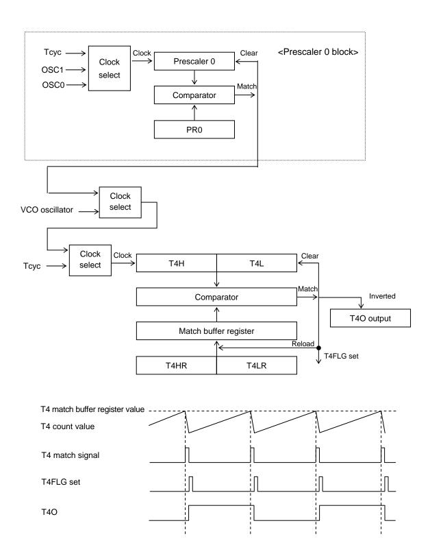
Figure 3.20.1 Timer 4 Block Diagram
