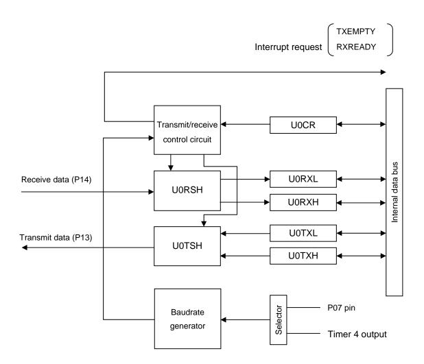
Figure 3.23.1 UART0 Block Diagram
