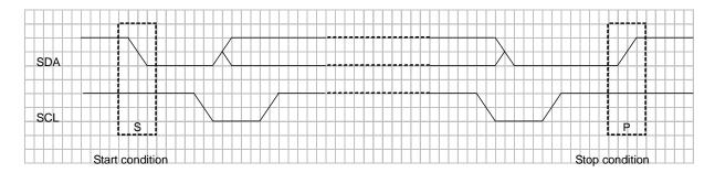
Figure 3.31.3 Start Condition and Stop Condition
