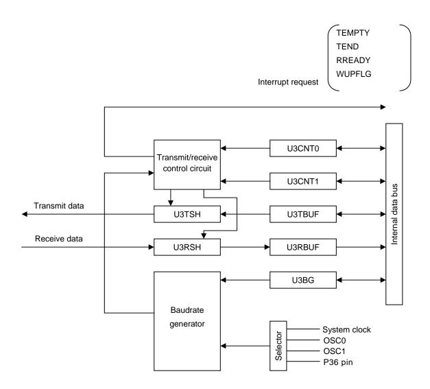
Figure 3.25.1 UART3 Block Diagram
