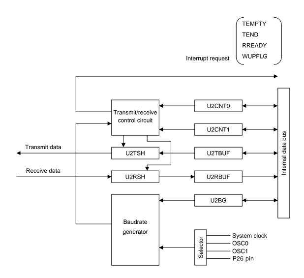
Figure 3.24.1 UART2 Block Diagram
