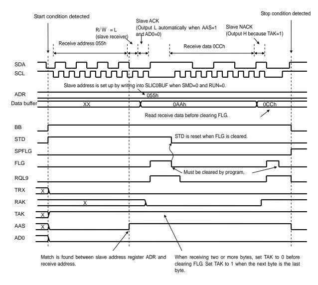
Figure 3.31.5 I<sup>2</sup>C Mode 1-byte Reception Timing Diagram
