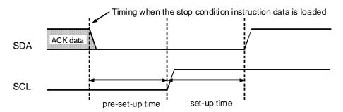
Figure 3.29.7 Stop Condition Generation Timing
