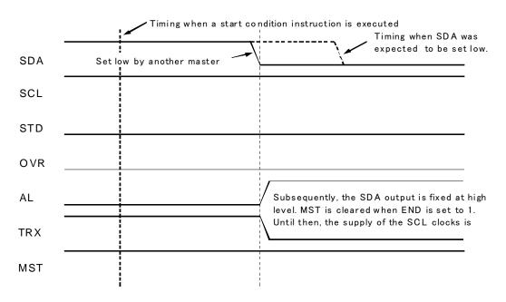
Figure 3.29.10 Arbitration Lost During Start Condition Generation <2>
