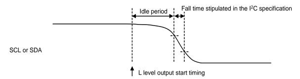
Figure 3.29.2 I<sup>2</sup>C Port Falling Waveform
