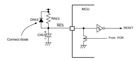
Figure 4-6-8: External POR reset circuit configuration example
