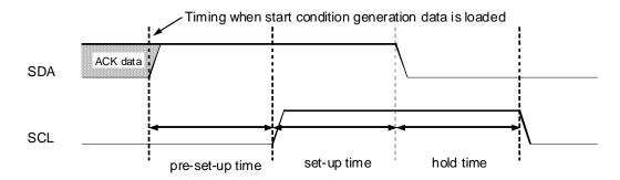
Figure 3.30.6 Restart Condition Generation Timing
