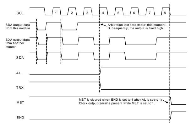
Figure 3.29.8 Arbitration Lost During Data Transfer
