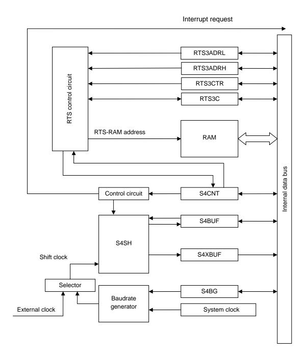
Figure 3.28.1 SIO4 Block Diagram
