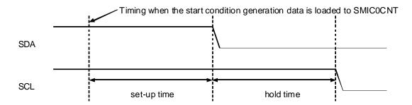
Figure 3.29.5 Start Condition Generation Timing Diagram
