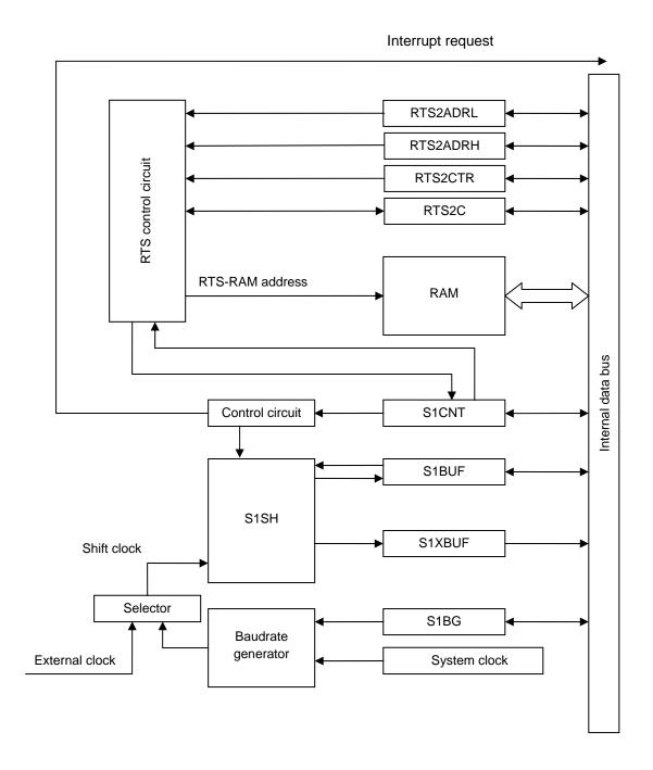
Figure 3.27.1 SIO1 Block Diagram
