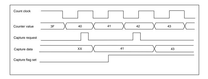
Figure 3.18.1 Capture Timing
