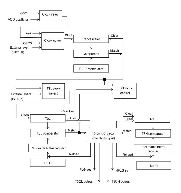
Figure 3.19.1 Timer 3 Block Diagram
