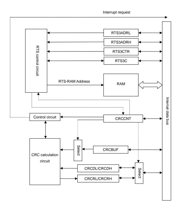
Figure 3.35.1 RTS Block Diagram
