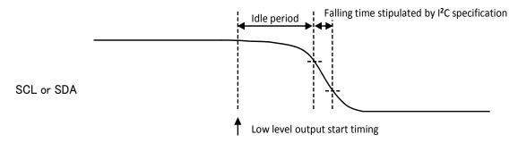
Figure 3.31.2 I<sup>2</sup>C Port Falling Edge Waveform
