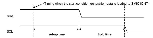
Figure 3.30.5 Start Condition Generation Timing Diagram
