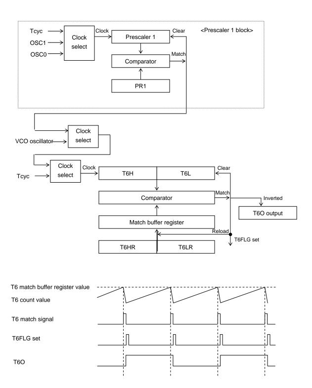
Figure 3.21.1 Timer 6 Block Diagram
