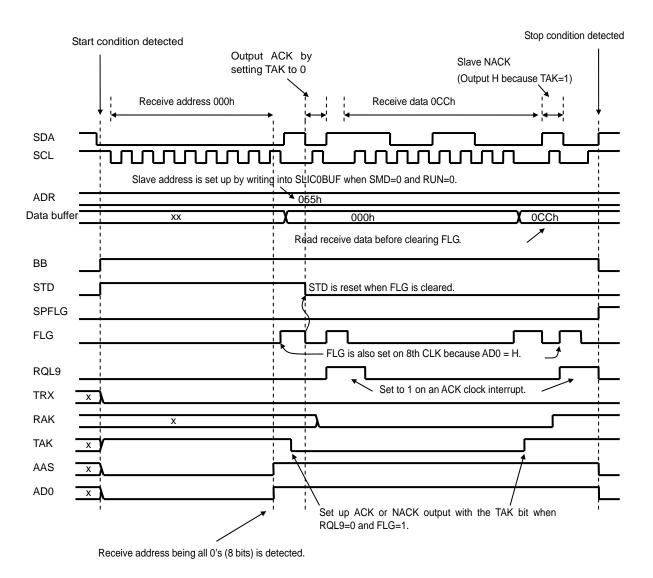
Figure 3.31.6 1<sup>2</sup>C Mode 1-byte Reception Timing Diagram (General Call)
