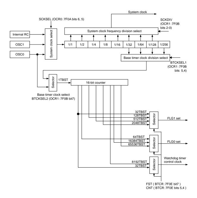
Figure 3.22.1 Base Timer Block Diagram
