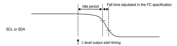
Figure 3.30.2 I<sup>2</sup>C Port Falling Waveform
