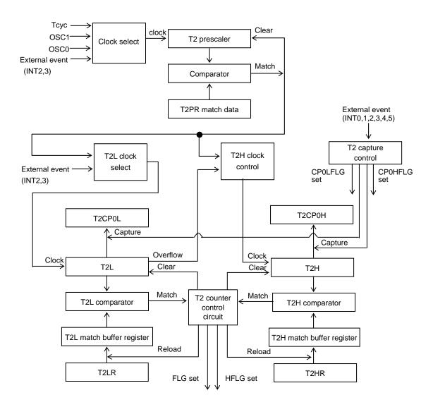
Figure 3.18.2 Timer 2 Block Diagram
