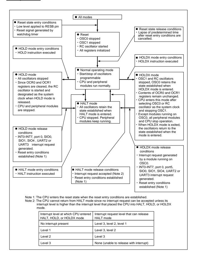
Figure 4.3.1 Standby Mode State Transition Diagram
