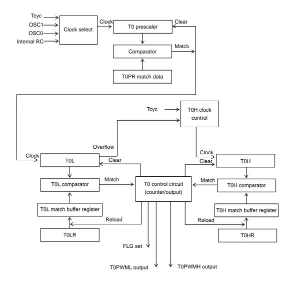
Figure 3.16.1 Timer 0 Block Diagram
