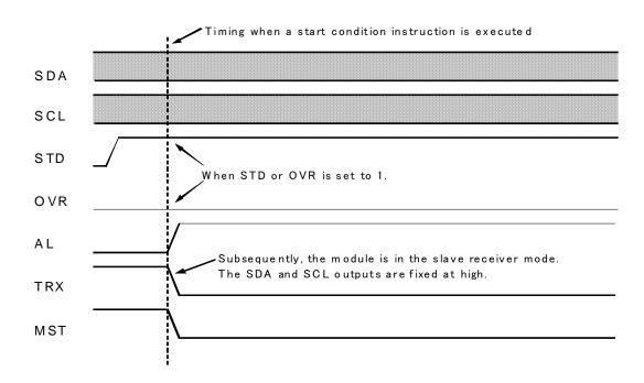
Figure 3.29.9 Arbitration Lost During Start Condition Generation <1>
