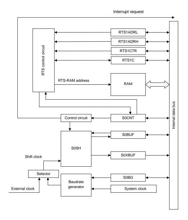
Figure 3.26.1 SIO0 Block Diagram
