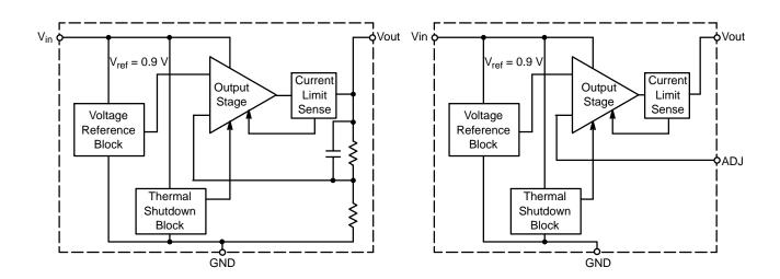
Figure 3. Block Diagram, Fixed Output
