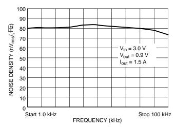
Figure 17. Noise Density vs. Frequency
