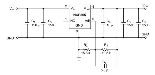
Figure 20. Schematic of NCP565 Typical Application Circuit
