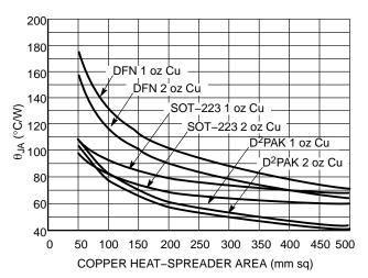
Figure 25. Thermal Resistance
