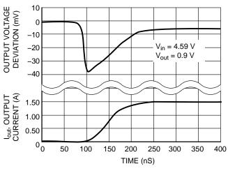
Figure 13. Load Transient from 10 mA to 1.5 A
