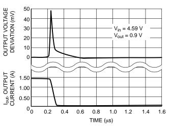
Figure 16. Load Transient from 1.5 A to 10 mA
