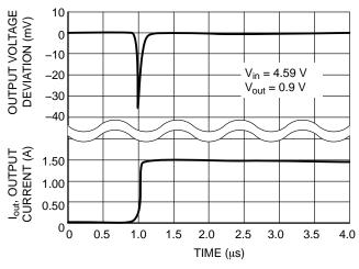
Figure 14. Load Transient from 10 mA to 1.5 A
