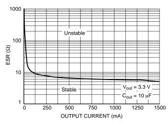
Figure 12. Output Capacitor ESR Stability vs.
