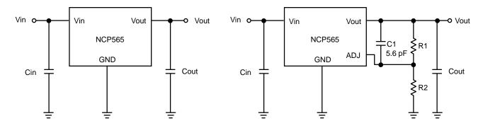
Figure 1. Typical Application Schematic, Fixed Output
