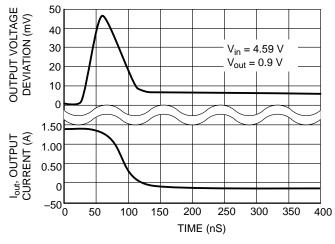
Figure 15. Load Transient from 1.5 A to 10 mA
