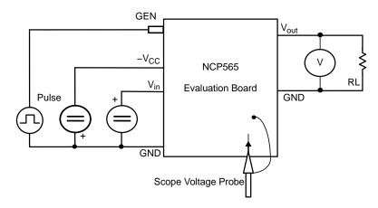
Figure 19. Schematic for Transient Response Measurement
