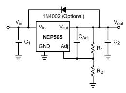
Figure 24. Protection Diode for Large Output Capacitors
