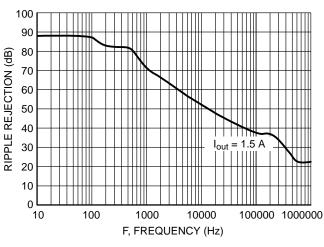
Figure 11. Ripple Rejection vs. Frequency
