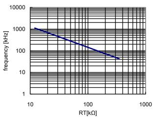
Figure 7. GATE frequency vs RT
