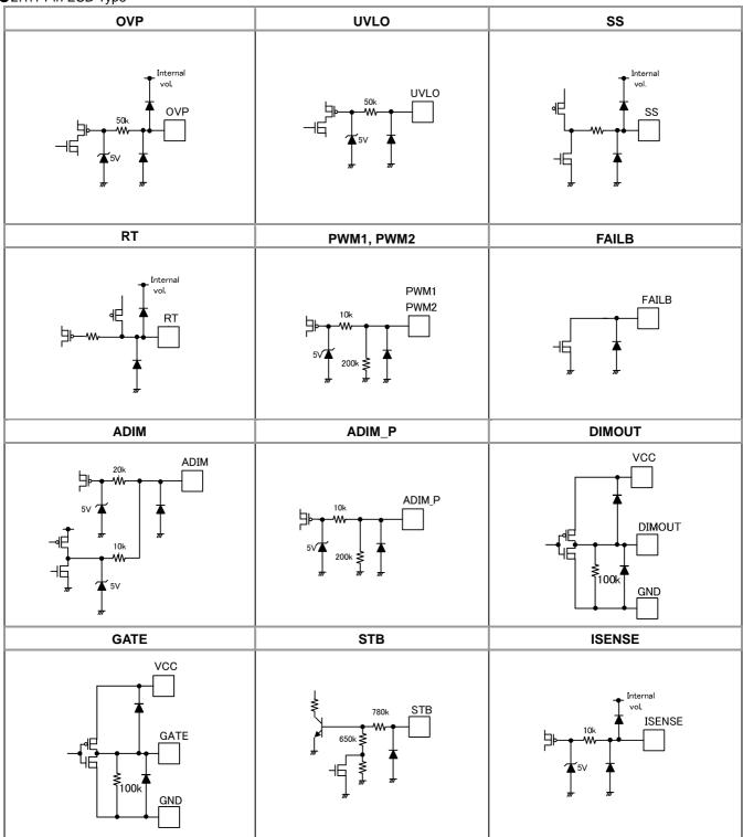
Figure 4-1. Internal equivalent circuit
