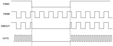
Figure 11. PWM pin function
