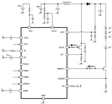
Figure 16. The basic application circuit example
