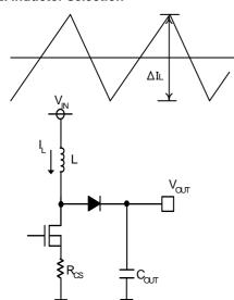
The inductor value affects the input ripple current. The equality in the section 3.5.1 is as following.
