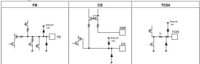
Figure 4-2. Internal equivalent circuit
