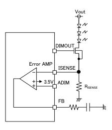
Figure 24. the example of LED current setting
