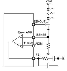
Figure 14. ISENSE pin circuit
