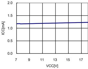
Figure 6. Operating current (ICC) vs VCC
