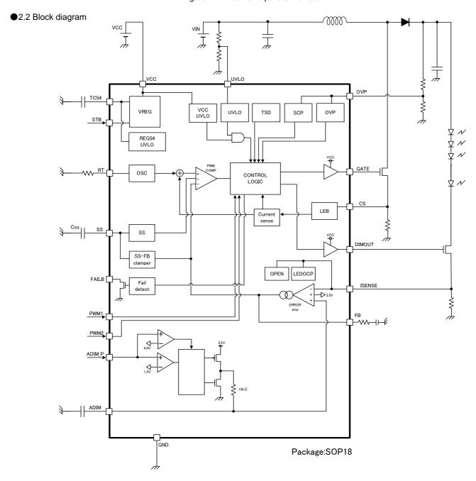
Figure 5. Block diagram
