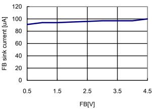
Figure 8. FB sink current vs FB voltage
