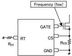
Figure 25. RT pin setting example
