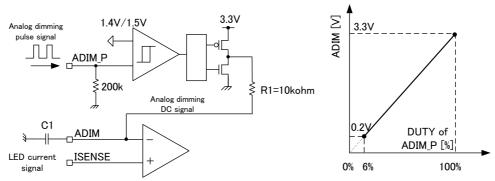
Figure 12. Analog dimming function and character
