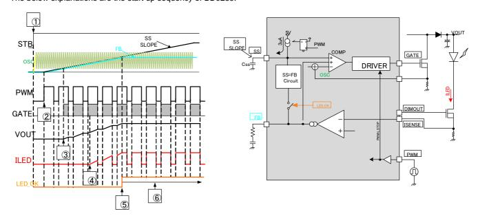
Figure 21. the turn-on waveform
