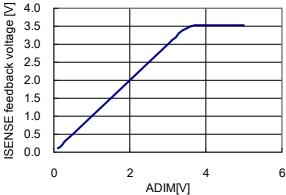
Figure 10. ISENSE feedback voltage vs ADIM
