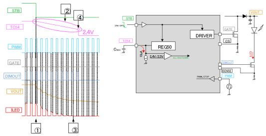
Figure 23. the shutdown waveform and circuit
