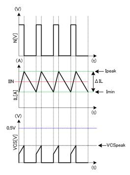
Figure 28. Coil current waveform
