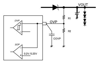
Figure 27. OVP/SCP setting example
