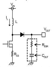
Figure 30. the output capacitor circuit
