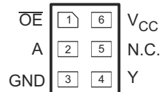
图 5-1. DBV package 5-pin SOT-23 (Top View)
