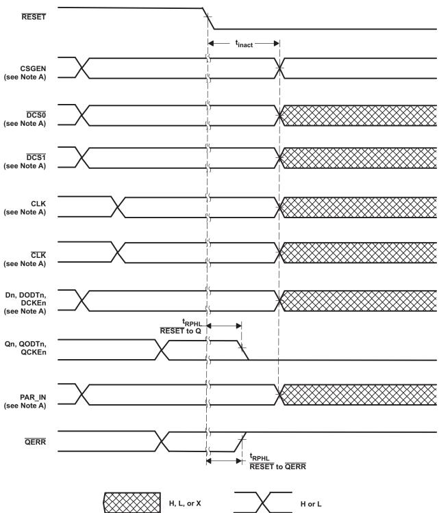
A. After RESET is switched from high to low, all data and clock input signals must be held at logic levels (not floating) for a minimum time of t<sub>inact</sub> max, to avoid a false error.
