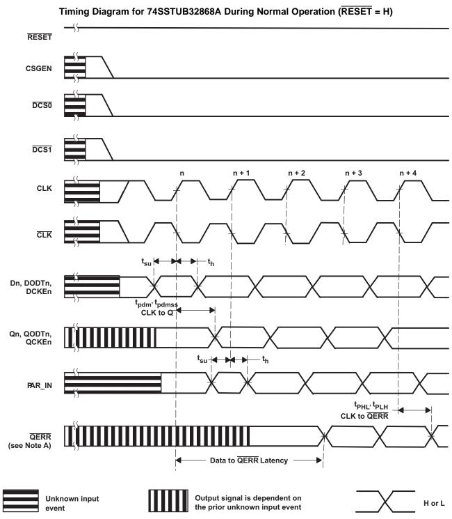
A. If the data is clocked in on the n-clock pulse, the QERR output signal is generated on the n + 2 clock pulse, and it is valid on the n + 3 clock pulse. If an error occurs and the QERR output is driven low, it stays latched low for a minimum of two clock cycles or until RESET is driven low.
