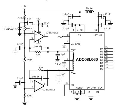
A. Driving the reference to force desired values requires driving with a low impedance source.
