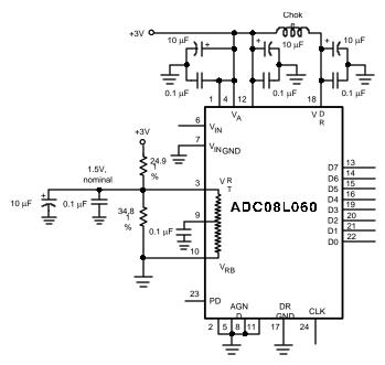
A. Because of the ladder and external resistor tolerances, the reference voltage of this circuit can vary too much for some applications.
