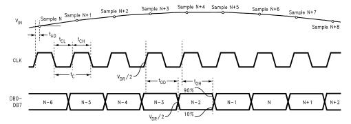
Figure 1. ADC08L060 Timing Diagram
