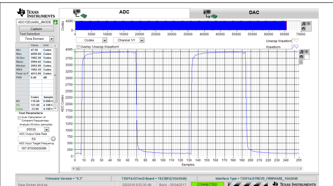
图 8-7. 40-MHz, Square-Wave Time Domain for 5-GSPS, Single-Channel Oscilloscope
