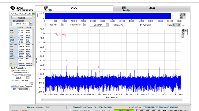
图 8-9. 200-MHz, Sine-Wave Frequency Domain (FFT) for 5-GSPS, Single-Channel Oscilloscope
