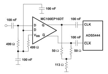
Figure 18. Differential Clock Using PECL Logic
