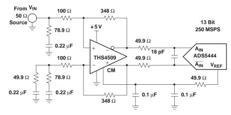
Figure 15. Using the THS4509 with the ADS5444
