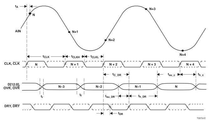
Figure 1. Timing Diagram
