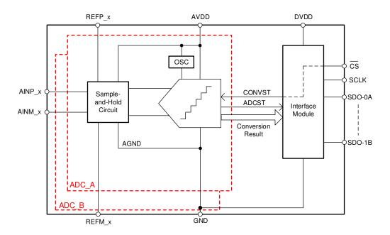
Figure 7-1. Converter Modules
