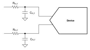
Figure 8-1. Charge-Kickback Filter
