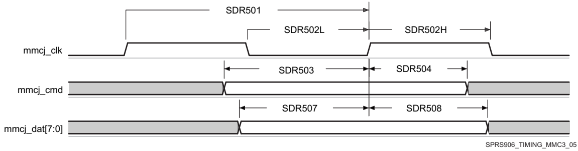
图 7-89. MMC/SD/SDIOj in - High Speed SDR50 - Receiver Mode
