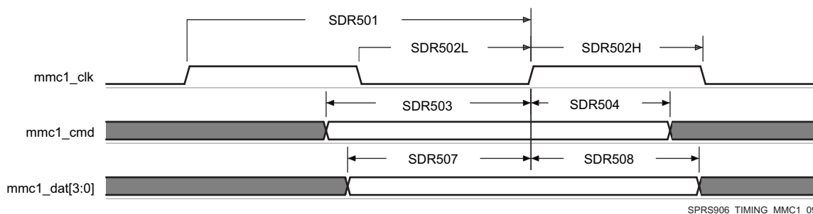
图 7-68. MMC/SD/SDIO in - High Speed SDR50 - Receiver Mode
