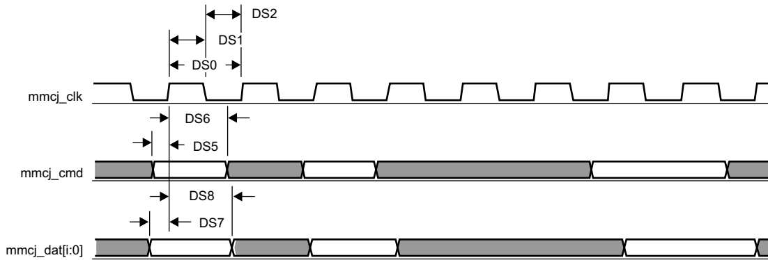
图 7-81. MMC/SD/SDIOj in - Default Speed - Receiver Mode
