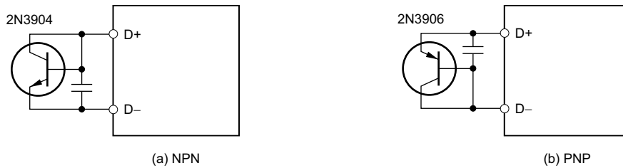
Figure 88. Remote Temperature Sensor Using Transistor
