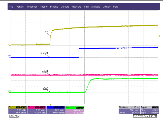
图 10-16. Charge Profile with Battery Simulator - STAT
