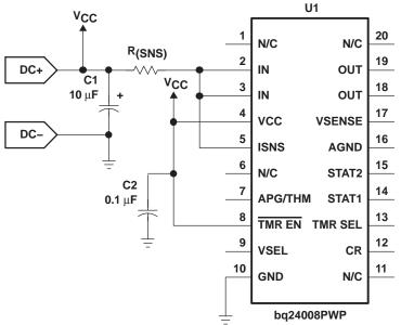
Figure 19. Current Sensing Circuit
