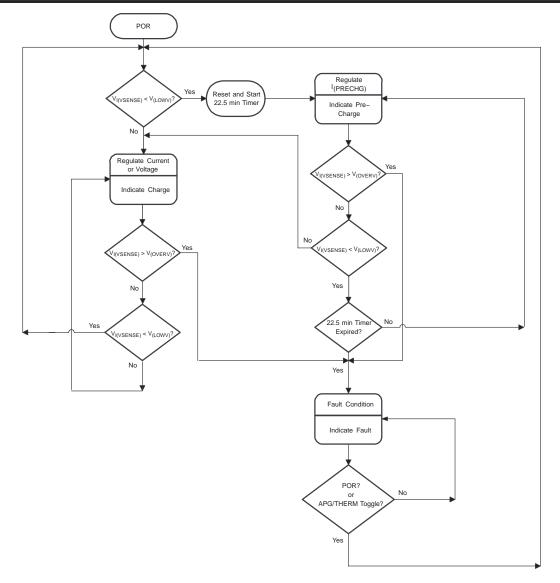
Figure 15. Operational Flow Chart With the Charge Timers Disabled (TMR EN = 1)
