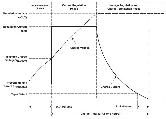
Figure 13. Typical Charge Profile
