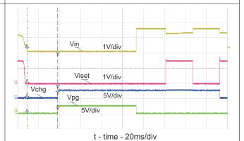
$V_{\text{IN}}$  swept from 5V to 3.9V to 5V
