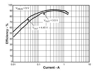
Figure 25. Charger Efficiency
