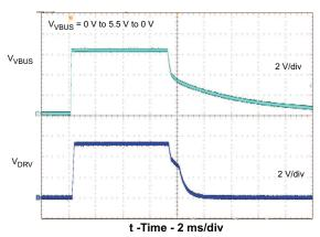
Figure 22. DRV Startup/Shutdown
