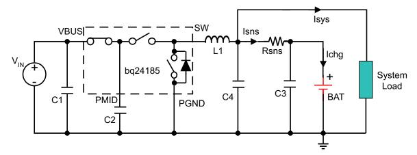
Figure 39. System Load Before Sensing Resistor
