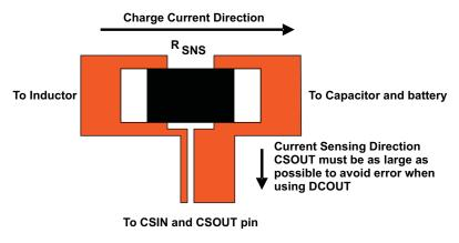
Figure 41. Sensing Resistor PCB Layout
