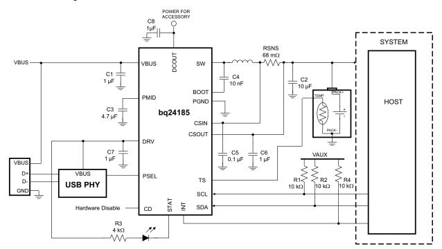
Figure 3. I<sup>2</sup>C Controlled 1-Cell USB Charger Application Circuit
