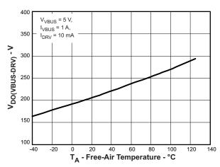
Figure 21. DRV Dropout vs T<sub>A</sub>
