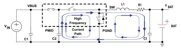
Figure 40. High Frequency Current Path
