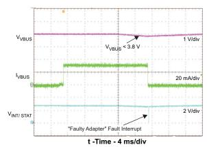
Figure 7. Faulty Adapter Detection
