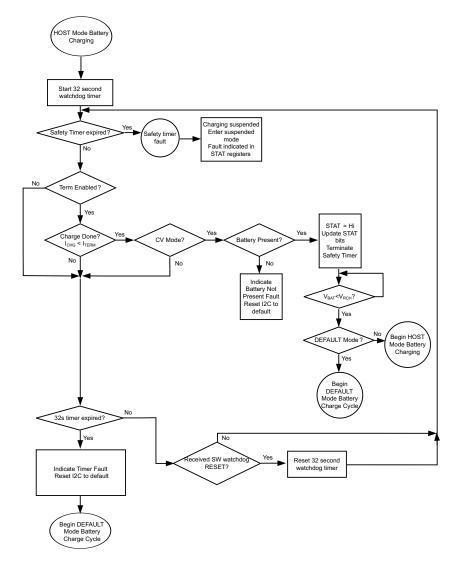
Figure 29. Host Mode Charging Process
