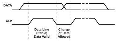
Figure 35. Bit Transfer on the Serial Interface
