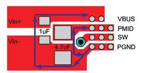
Figure 42. Input Capacitor Position and PCB Layout Example
