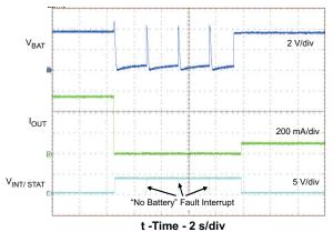
Figure 5. Battery Insertion/Removal
