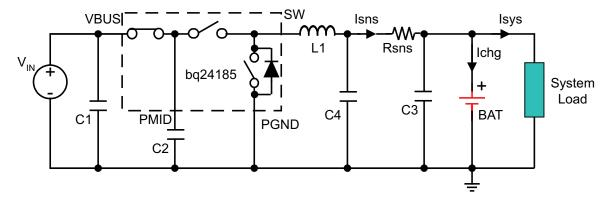
Figure 38. System Load After Sensing Resistor
