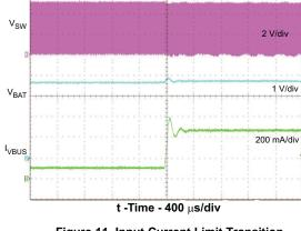
Figure 11. Input Current Limit Transition USB100 to USB500
