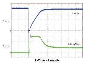
Figure 18. Hotplug 1000µF Capacitor into DCOUT
