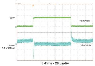
Figure 23. DRV Load Transient
