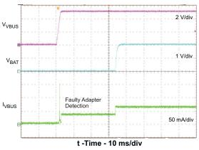
Figure 14. Startup Into Default Mode No Battery Connected
