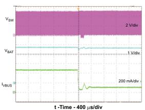
Figure 10. Input Current Limit Transition USB500 to USB100
