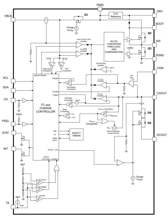
Figure 1. Simplified Block Diagram (Charge Mode, OPA\_MODE = 0)
