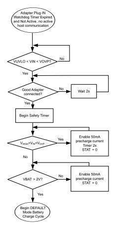
Figure 26. Startup on Adapter Plug-In in DEFAULT Mode
