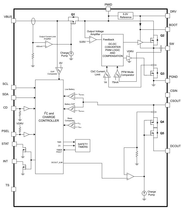
Figure 2. Simplified Block Diagram (Boost Mode, OPA\_MODE = 1)
