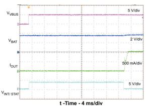
Figure 6. PWM Charging Waveforms
