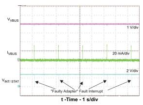
Figure 8. Faulty Adapter Detection (Showing Continuous Detection)
