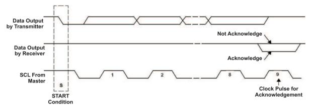
Figure 36. Acknowledge on the I2C Bus
