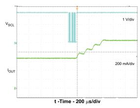
Figure 13. Charge Current Transition 550mA to 1.05A Using I<sup>2</sup>C
