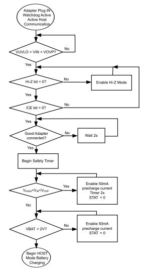
Figure 27. Startup on Adapter Plug-In in Host-Controlled Mode
