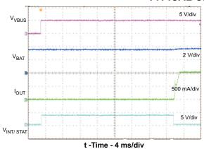
Figure 4. Adapter Insertion
