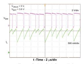
Figure 9. Cycle by Cycle Current Limit
