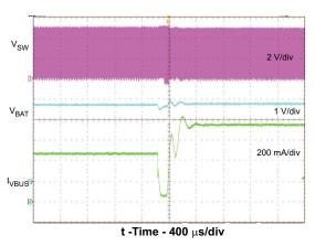
Figure 12. Input Current Limit Transition USB500 to 750mA
