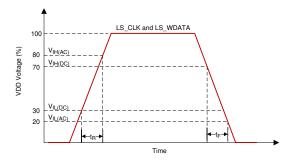
Figure 6-3. LPSDR Input Slew Rate
