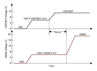
A. Refer to Table 9-1 for V<sub>OFFSET</sub> and V<sub>BIAS</sub> supply voltage levels during power-up sequence delay.
