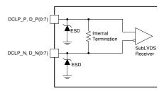
Figure 6-11. SubLVDS Equivalent Input Circuit
