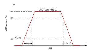
Figure 6-4. LPSDR Input Slew Rate
