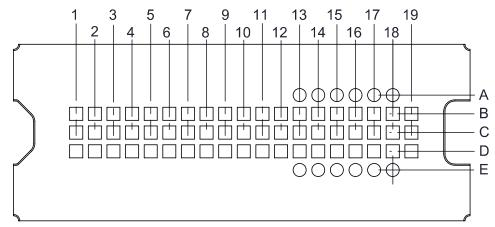
Figure 5-1. FQK Package 57-Pin LGA (Bottom View)
