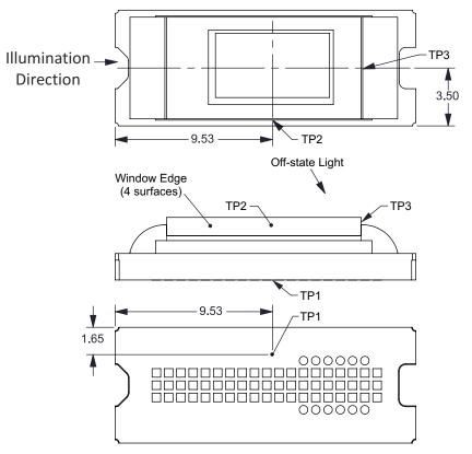
Figure 7-1. DMD Thermal Test Points
