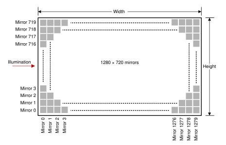
Figure 6-16. Micromirror Array Physical Characteristics
