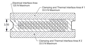
Figure 6-15. System Interface Loads
