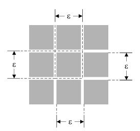
Figure 6-17. Mirror (Pixel) Pitch
