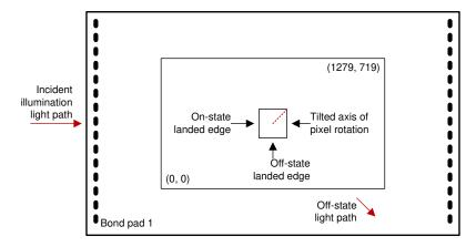
Figure 6-18. Landed Pixel Orientation and Tilt
