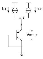
Figure 11. Temperature Measurement Theory
