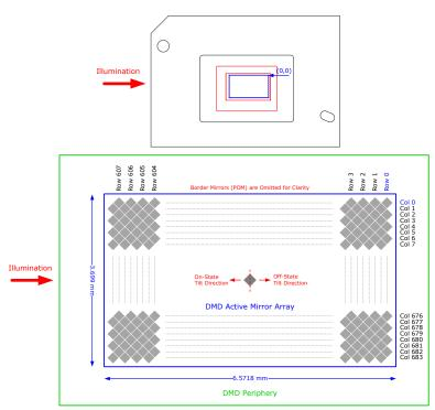
Figure 7. Micromirror Array Physical Characteristics
