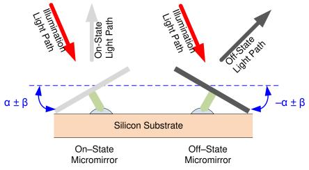
Figure 9. Micromirror Tilt Angle
