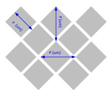
Figure 8. Mirror (Pixel) Pitch
