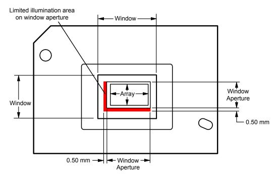
Figure 1. Illumination Overfill Diagram
