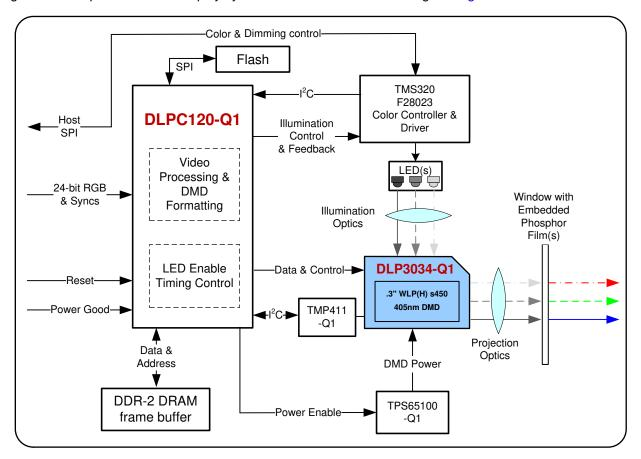
Figure 18. DLP3034-Q1 Reference Design Block Diagram
