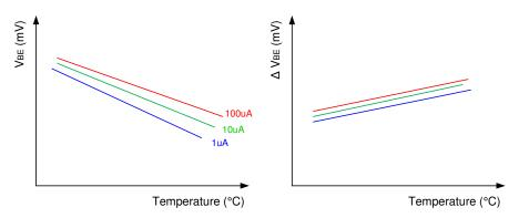
Figure 12. Example of Delta VBE vs Temperature
