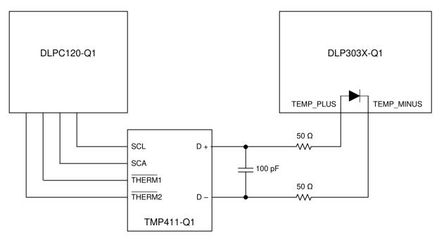
Figure 10. Temperature Sense Diode Typical Circuit Configuration
