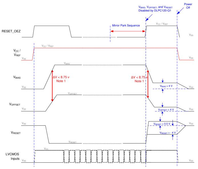
(1) ±8.75-V delta, ΔV, shall be considered the max operating delta between V<sub>BIAS</sub> and V<sub>OFFSET</sub>. Customers may find that the most reliable way to ensure this is to power V<sub>OFFSET</sub> prior to V<sub>BIAS</sub> during power up and to remove V<sub>BIAS</sub> prior to V<sub>OFFSET</sub> during power down.
