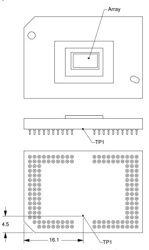
Figure 17. Thermocouple Locations
