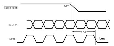
Figure 12. DS90CR482 (Receiver) Power Down Delay
