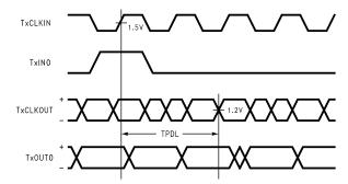
Figure 7. DS90CR481 (Transmitter) Propagation Delay - Latency
