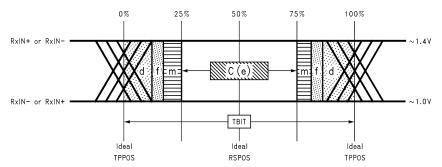
C — Setup and Hold Time (Internal data sampling window) defined by Rspos (receiver input strobe position) min and max
