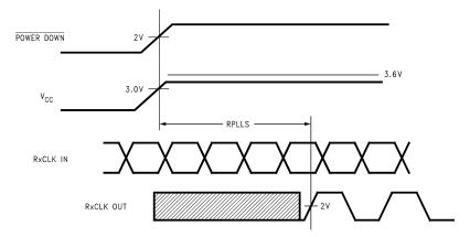
Figure 10. DS90CR482 (Receiver) Phase Lock Loop Set Time
