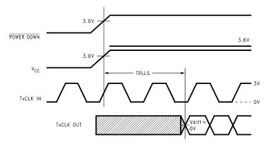
Figure 9. DS90CR481 (Transmitter) Phase Lock Loop Set Time
