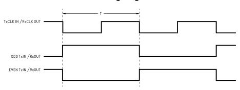
(1) The worst case test pattern produces a maximum toggling of digital circuits, LVDS I/O and CMOS/TTL I/O.
