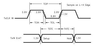
Figure 5. DS90CR481 (Transmitter) Setup/Hold and High/Low Times
