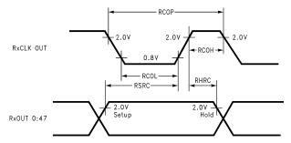
Figure 6. DS90CR482 (Receiver) Setup/Hold and High/Low Times
