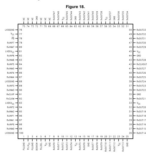
Figure 19. Receiver - DS90CR482 - TQFP - Top View
