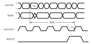
Figure 8. DS90CR482 (Receiver) Propagation Delay - Latency
