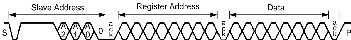
Figure 35. Serial Control Bus: WRITE
