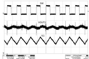
图 8-4. Typical Switching Waveform ( $V_{IN}$  = 24 V,  $I_{OUT}$  = 100 mA)
