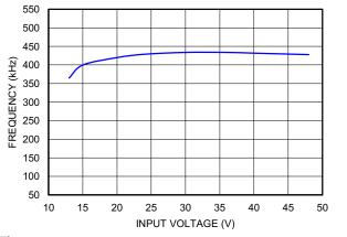
图 8-3. Frequency versus Input Voltage (I<sub>OUT</sub> = 100 mA)
