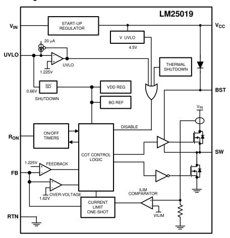
图 7-1. Functional Block Diagram
