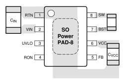
图 10-1. Placement of Bypass Capacitors
