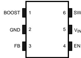
Package DDC (R-PDSO-G6) 6-Lead SOT Top View
