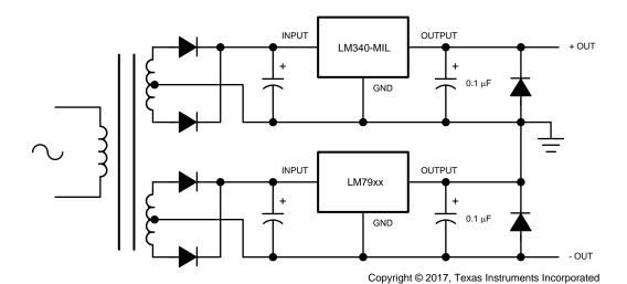
Figure 26. Device Used With Negative Regulator LM79xx
