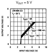
Figure 19. Output Voltage vs Input Voltage
