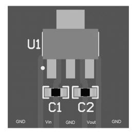
Figure 28. Layout Example SOT-223
