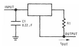
$I_{OUT}$  = V2–3 / R1 +  $I_{Q}$   $\Delta I_{Q}$  = 1.3 mA over line and load changes.
