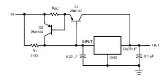
$\begin{aligned} R_{SC} &= 0.8 \ / \ I_{SC} \\ R1 &= \beta V_{BE(Q1)} \ / \ I_{REG\ Max} \left(\beta + 1\right) - I_{O\ Max} \end{aligned}$
