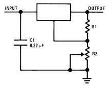
$V_{OUT} = 5 \text{ V} + (5 \text{ V/R1} + I_Q)$ R2 5 V/R1 > 3 I<sub>Q</sub>, load regulation (L<sub>r</sub>)  $\approx$  [(R1 + R2)/R1] (L<sub>r</sub> of LM340-MIL-5).
