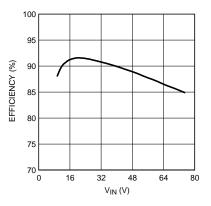
Figure 40. Efficiency vs. Input Voltage
