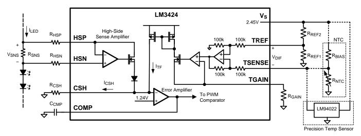
Figure 20. Thermal Foldback Circuitry
