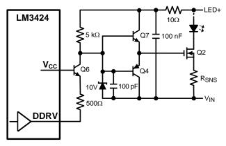
Figure 32. Buck-Boost Level-Shifted PWM Circuit
