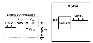
Figure 35. Timing Circuitry
