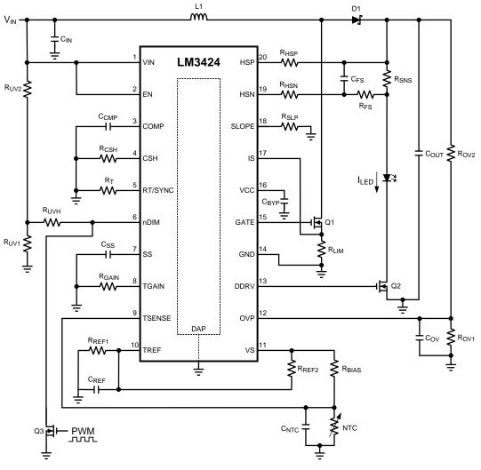
Figure 36. Boost Regulator ( $V_{IN} < V_O$ )
