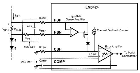
Figure 25. Compensation Circuitry
