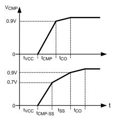
Figure 27. Start-up Waveforms
