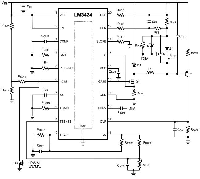
Figure 37. Buck Regulator ( $V_{IN} > V_O$ )
