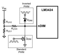
Figure 31. PWM Dimming Circuit
