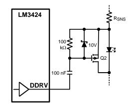
Figure 33. Buck Level-Shifted PWM Circuit
