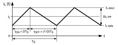
Figure 17. Ideal CCM Regulator Inductor Current i<sub>L</sub>(t)
