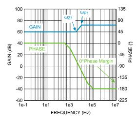
Figure 24. Uncompensated Loop Gain Frequency Response
