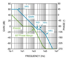
Figure 26. Compensated Loop Gain Frequency Response
