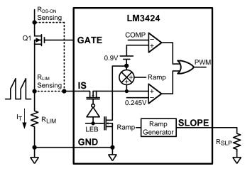
Figure 22. Current Sense / Current Limit Circuitry
