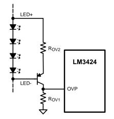
Figure 29. Floating Output OVP Circuitry
