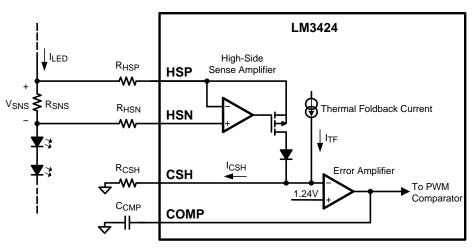
Figure 18. LED Current Sense Circuitry
