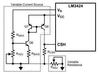
Figure 21. Analog Dimming Circuitry
