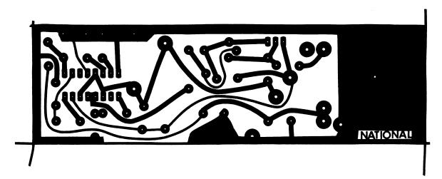
Figure 26. 5V, 1 Amp Switching Regulator, Foil Side
