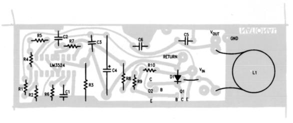
Figure 27. Stuffing Diagram, Component Side
