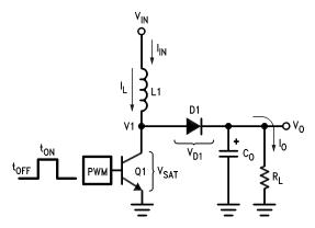
Figure 28. Basic Step-Up Switching Regulator
