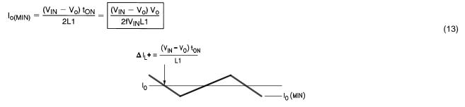
Figure 24. Inductor Current Slope in Step-Down Regulator
