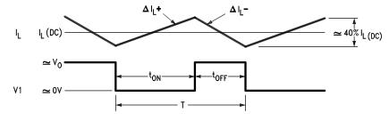
Figure 29. Relation of Switch Timing to Inductor Current in Step-Up Regulator
