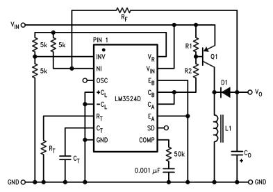
Figure 21. Boosted Current Polarity Inverter
