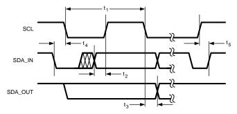
Figure 1. I<sup>2</sup>C-Compatible Interface Specifications
