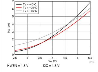
Figure 12. Standby Current vs Input Voltage
