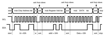
Figure 26. Write Cycle W = Write (SDA = "0") R = Read (SDA = "1") Ack = Acknowledge (SDA Pulled Down by Either Master or Slave) ID = Chip Address, 63h for LM3648
