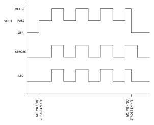
Figure 19. IR Mode with Boost
