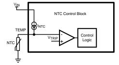
Figure 23. Temp Detection Diagram
