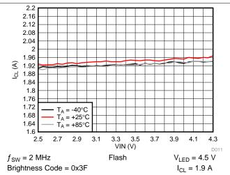
Figure 13. Inductor Current Limit vs Input Voltage
