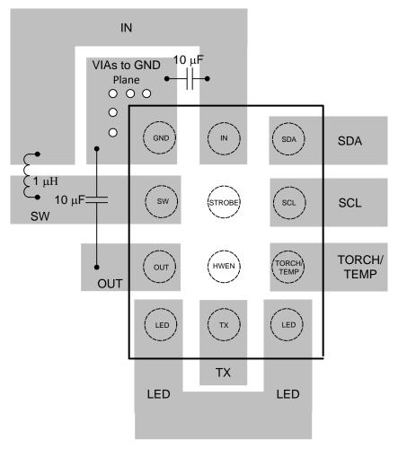
Figure 43. LM3648 Layout Example
