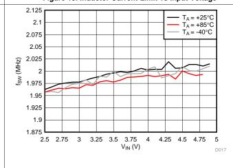
Figure 17. 2-MHz Switching Frequency vs Input Voltage
