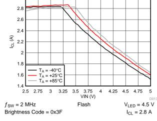
Figure 15. Inductor Current Limit vs Input Voltage
