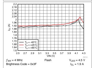
Figure 14. Inductor Current Limit vs Input Voltage
